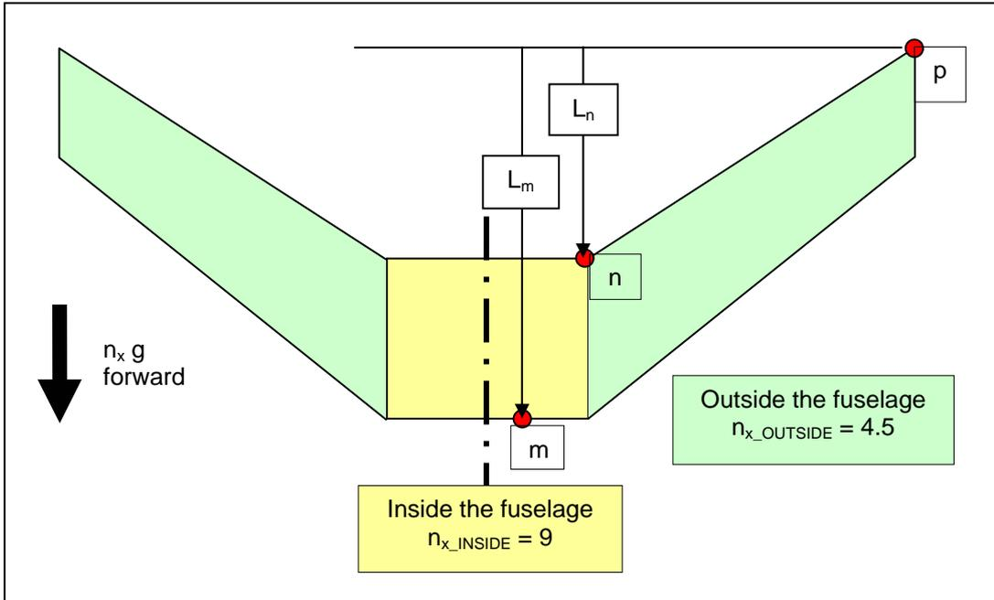
Figure a: Transmission of pressure from a fuel tank outside the fuselage and a fuel tank inside the fuselage (example with a forward load case)
