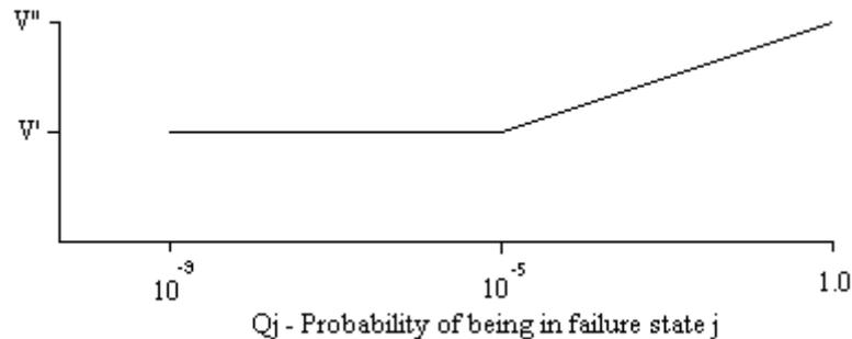
$V'$  = Clearance speed required for failure conditions as defined in sub-paragraph 4.1.1(ii)
