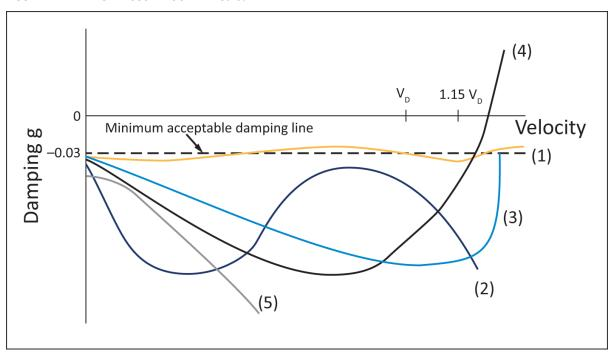
5.1.4. Analysis Considerations. Airframe aeroelastic stability analyses may be used to verify the design with respect to the structural stiffness, mass, fuel (including inflight fuel management), automatic flight control system characteristics, and altitude and Mach number variations within the design flight envelope. The complete aeroplane should be considered as composed of lifting surfaces and bodies, including all primary control surfaces which can interact with the lifting
