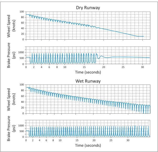
FIGURE 1. ANTI-SKID SYSTEM RESPONSE CHARACTERISTICS On-Off System
