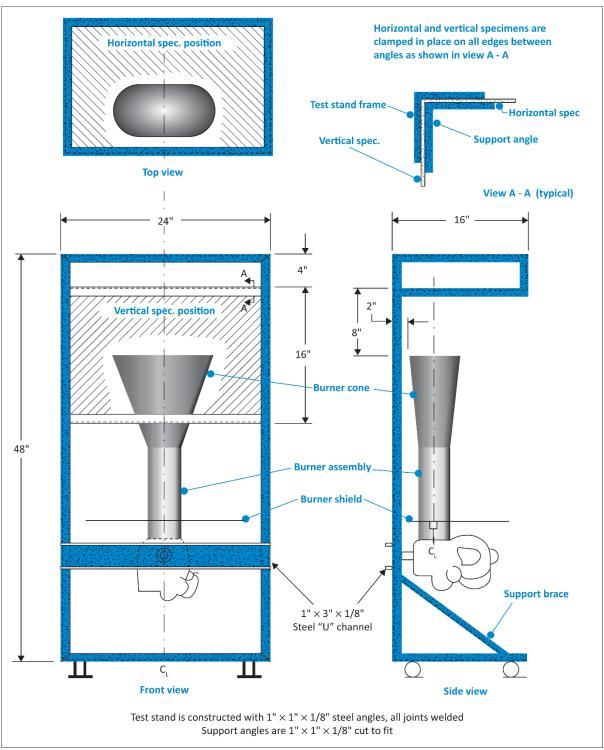
FIGURE 1 TEST APPARATUS FOR HORIZONTAL AND VERTICAL MOUNTING
