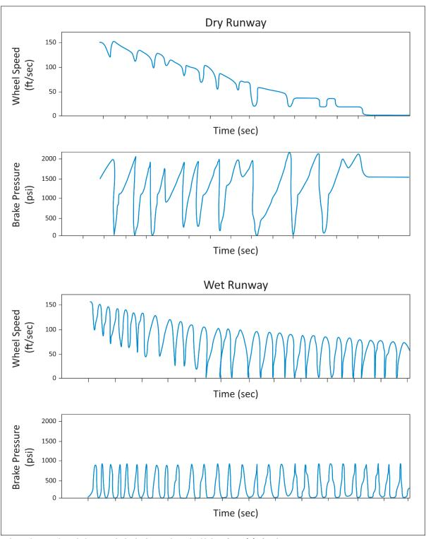
FIGURE 2. ANTI-SKID SYSTEM RESPONSE CHARACTERISTICS Quasi-Modulating System
