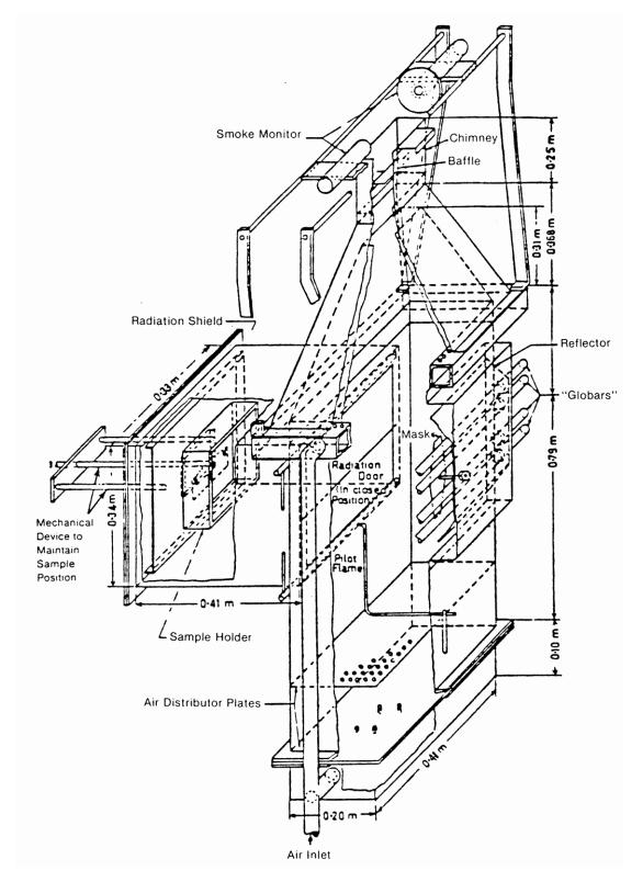
FIGURE 1. RELEASE RATE APPARATUS
