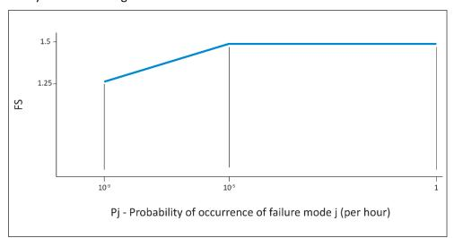
Figure 2 Factor of safety for continuation of flight
