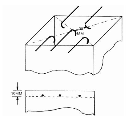
FIGURE 5. THERMOCOUPLE POSITION
