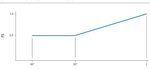
Figure 3: Factor of safety for continuation of flight
