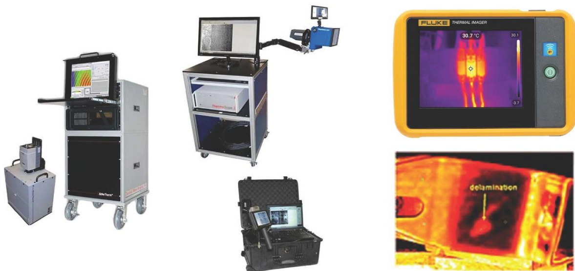
Figure 53 — Portable thermographic test equipment, potentially including an image evaluation system
