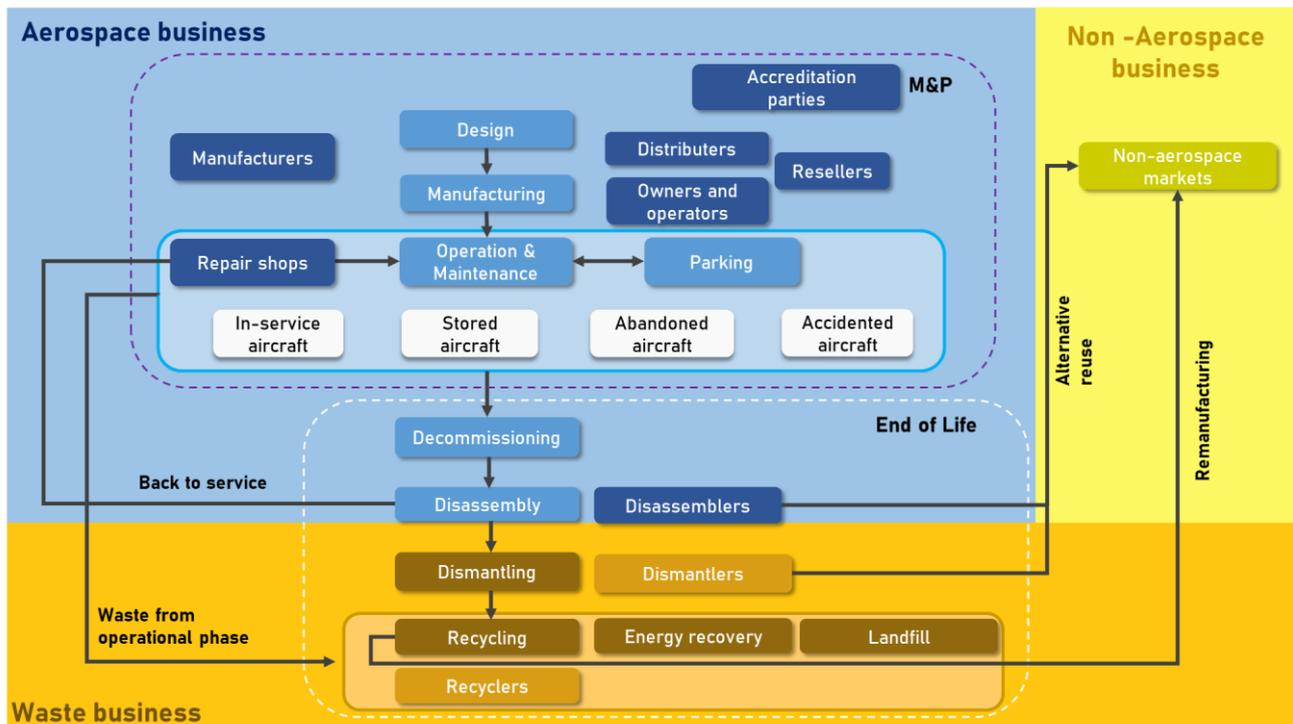
Figure 1. Main areas and units of the aircraft lifecycle
