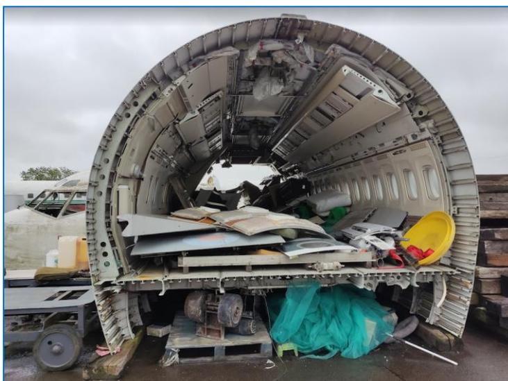
Figure 28. Aircraft section under dismantling. (Envisa, 2022)
