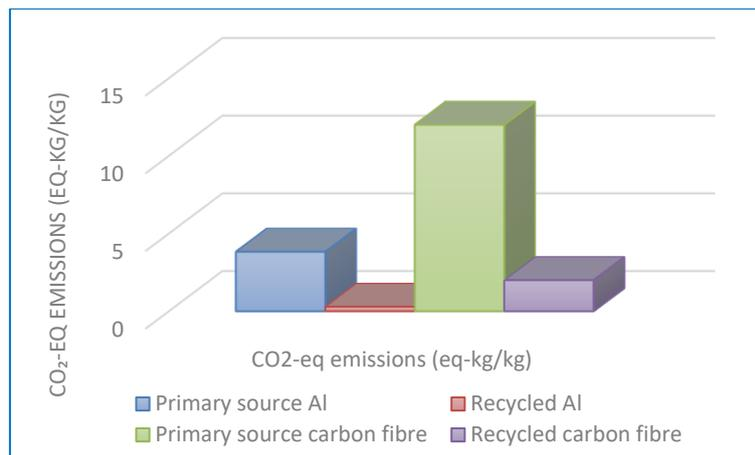
Figure 50. GHG savings from the use of recycled Al and carbon fibre (Data from Asmatulu et al., 2013)
