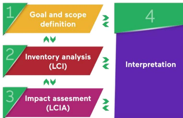
Figure 12. The LCA Process (ISO 14040)
