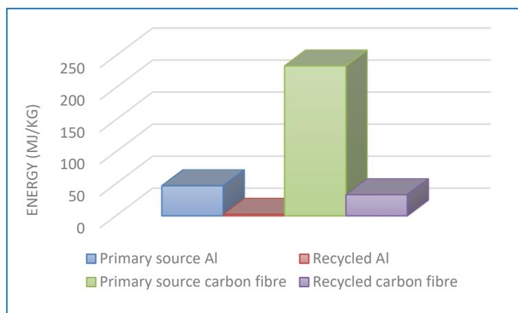
Figure 49. Energy savings from the use of recycled Al and carbon fibre (Data from Asmatulu et al., 2013)
