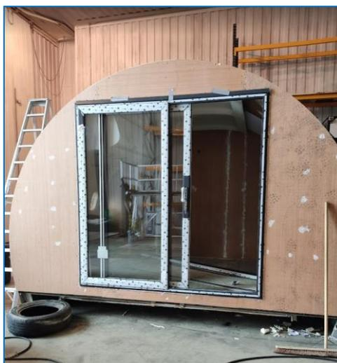
Figure 27. Aircraft cabin section undergoing a process to be reused as an office. (Envisa, 2022)
