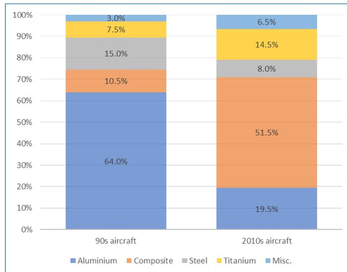
Figure 29. Representative aircraft material compositions in the 90s and 2010s (Wong et al. 2017)
