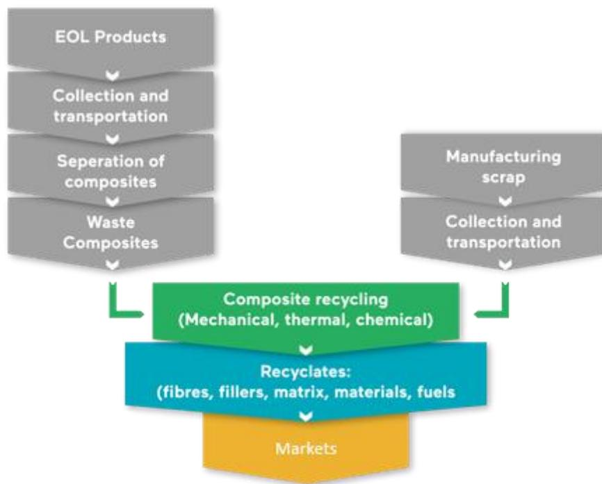
Figure 18. Structure of recycling system for composite materials. Yang et al (2012)<sup>48</sup>
