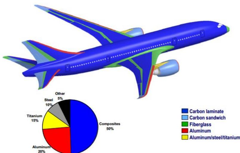
Figure 57. Aircraft materials mapping (Aimere project, 2014)
