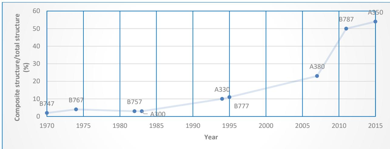
Figure 48. Share of composites in aircraft structure materials (values from Woidasky 2017<sup>105</sup>, Wong 2017<sup>106</sup>, and Towle 2004<sup>107</sup>)
