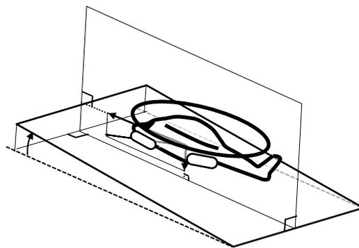
b) Water entry into inclined plane of stationary water, steepness range - zero to significant steepness ( $S_s$ )
