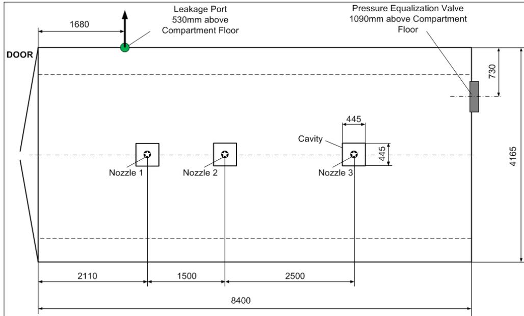
Figure 7: Position of Discharge Nozzles, Leakage Port, and Pressure Equalization Valve
