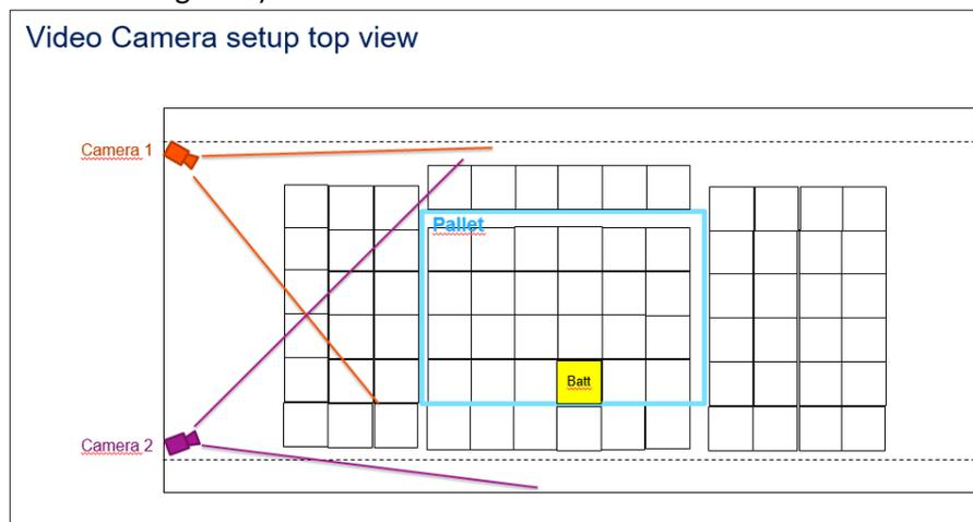
Figure 8: Video Camera instrumentation including field of view
