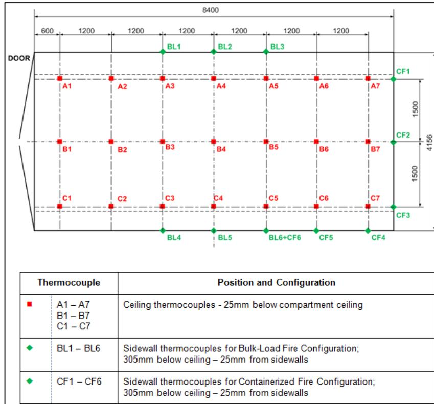
Figure 3. Thermocouple Position
