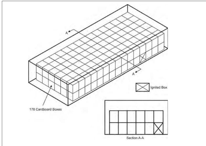
Figure 11: Arrangement of Cardboard Boxes as fire load for the Bulk load fire test of the Minimum Performance Standard for Aircraft Cargo Compartment Halon Replacement Fire Suppression Systems [2]
