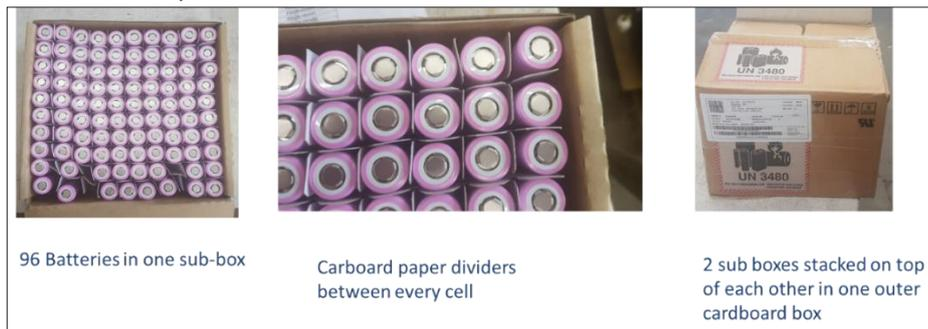
Figure 12: Manufacturer 1 cells packaging (the missing cells were taken to do some voltage checks)
