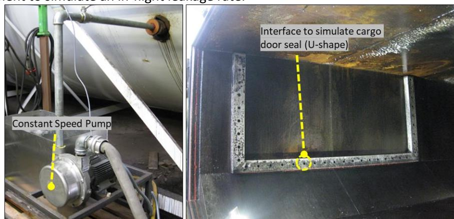
Figure 2. In-flight Leakage Simulation
