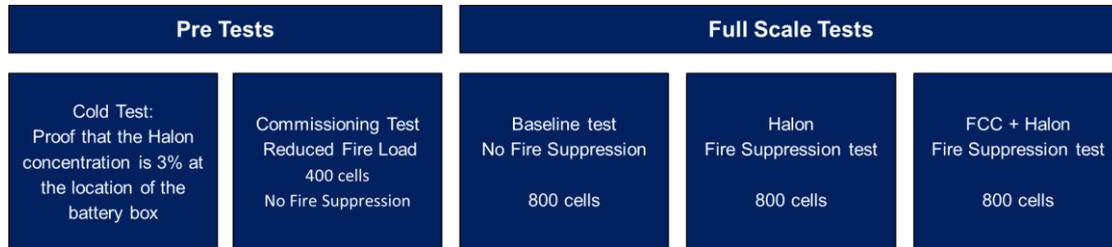
Figure 15: Test sequence for the Full scale test campaign.
