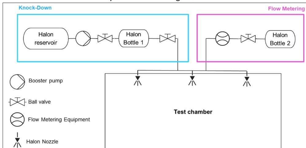
Figure 6: Schematic of the Halon Discharge system of the test chamber
