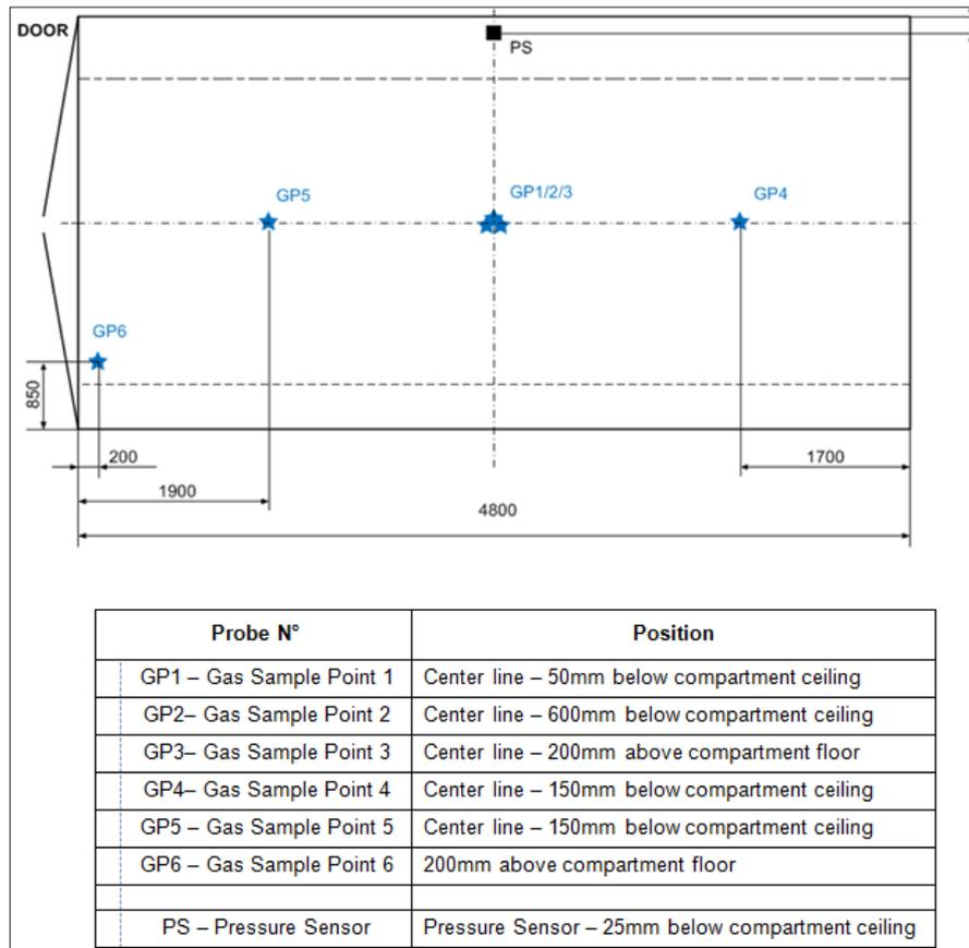
Figure 4. Position of Pressure Sensor and Gas Sample Points
