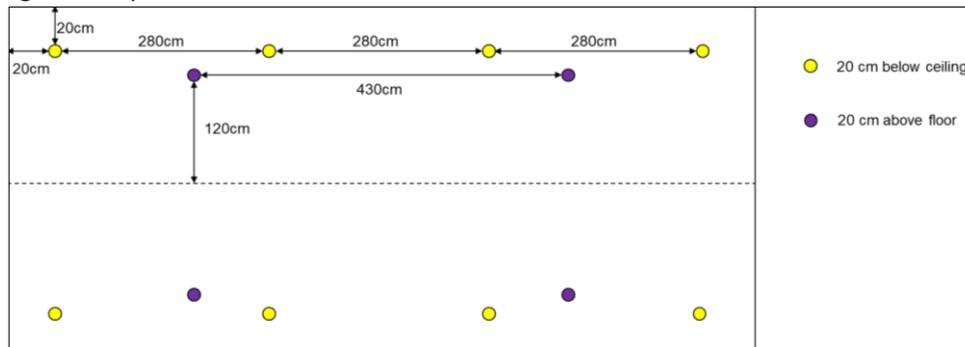
Figure 5: Halon Sensor location
