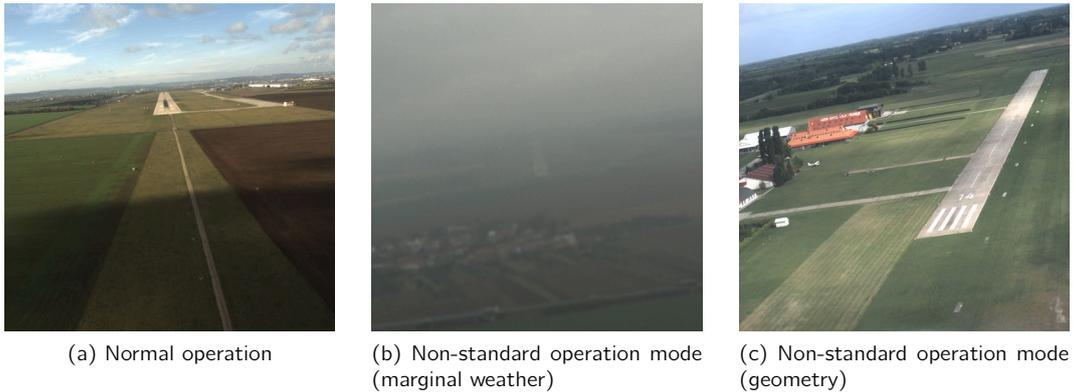
Figure 5.5: Domain bias due to inherently non-standard conditions. Example of a final approach to a runway (see Table 4.1, “ConOps”). (a): Most data is naturally coming from standard approaches under standard VFR conditions. (b, c): Operational domain shift due to marginal weather or non-standard approach angles, often irreducible due to the inherent danger of obtaining such data.
