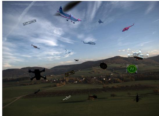
Figure 7.2: Augmentation of real data for the task of object detection: pictures of objects to be detected are pasted against a background. Note that some additions appear realistic (the aircraft), while some do not (the helipads).
