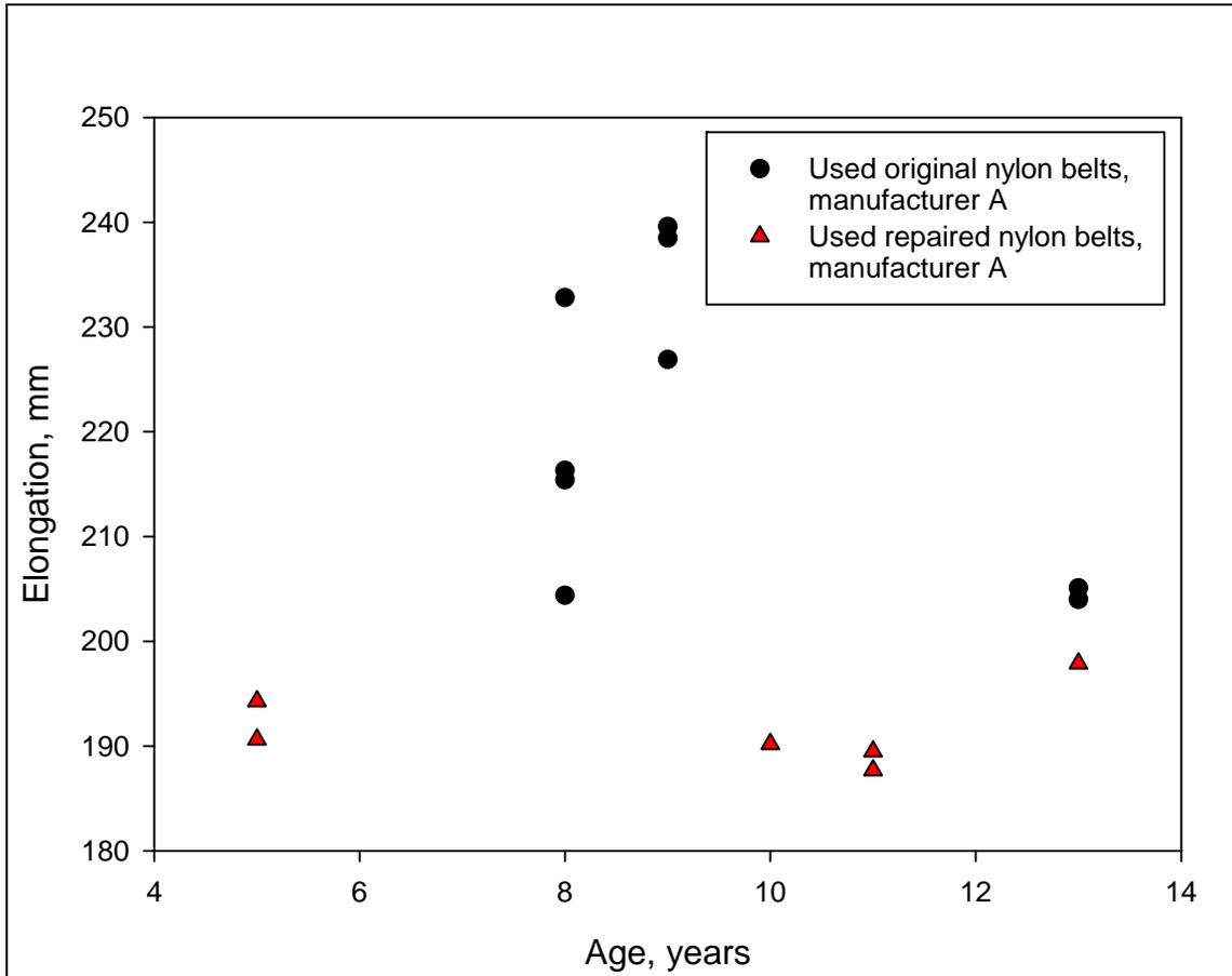
**Figure 8. Graph of elongation versus age for 2000lb belts at 18 kN static load**
