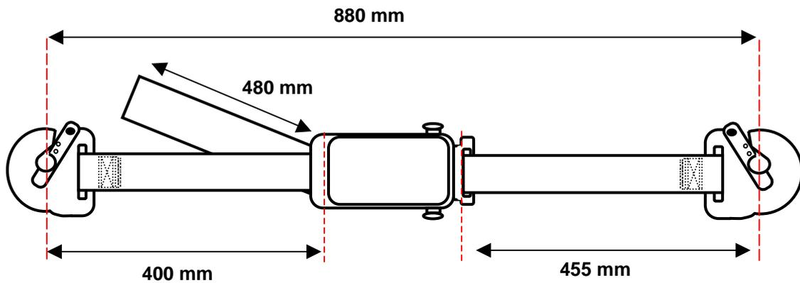
**Figure 2. Dimensions of 1340 mm belt in 16g Dynamic Test**
