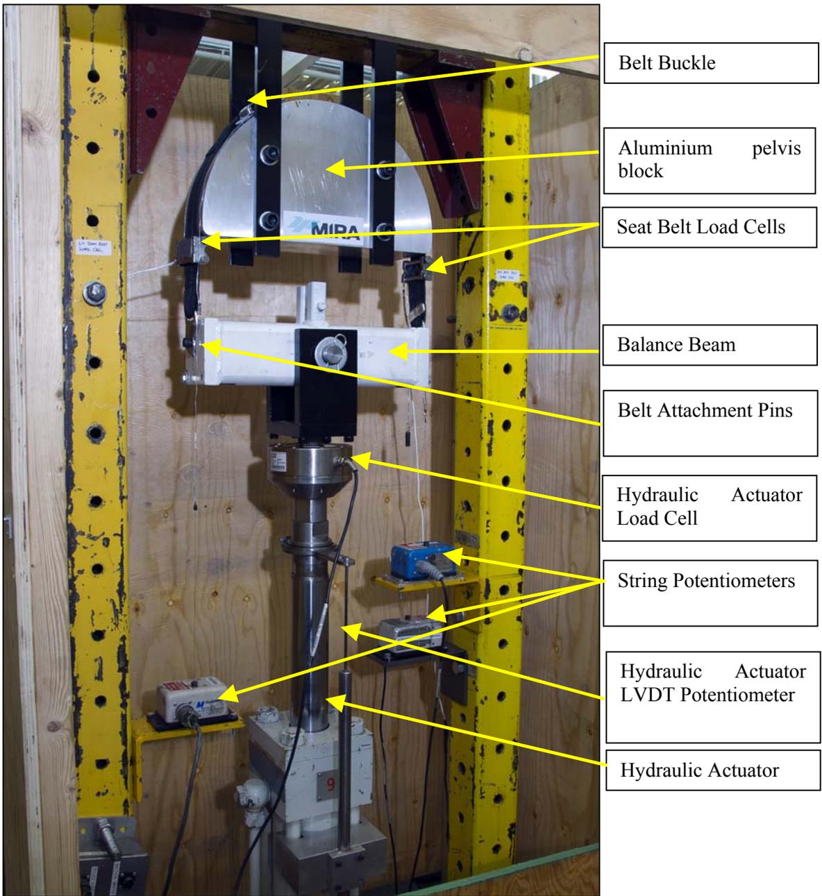
**Figure B.1.4 . Annotated photograph showing the location of the static test components and instrumentation**
