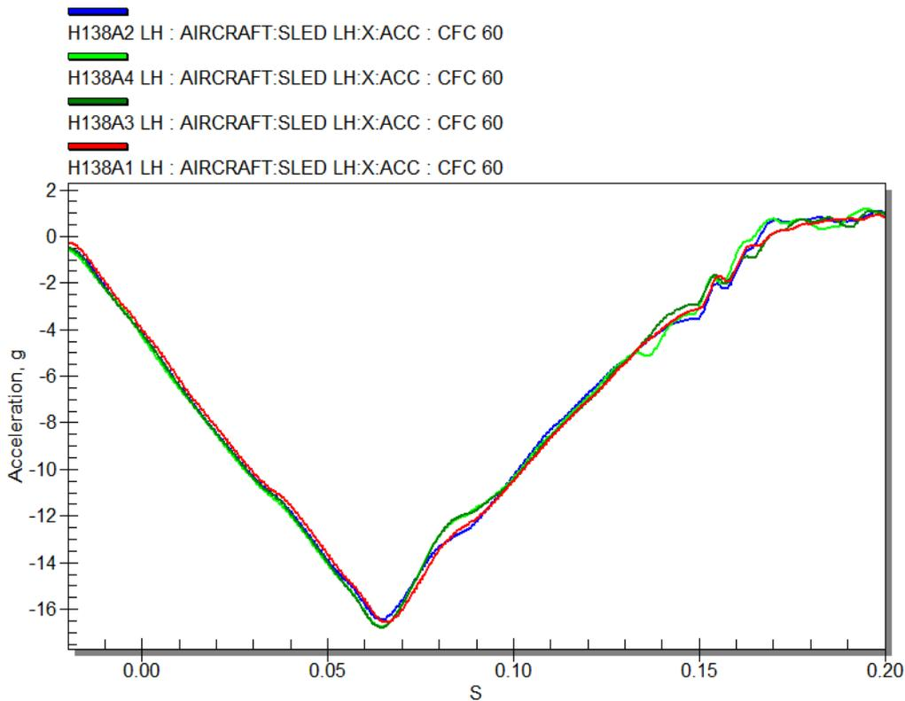
**Figure B.4.2. Acceleration profiles from the HyGe reverse accelerator sled.**
