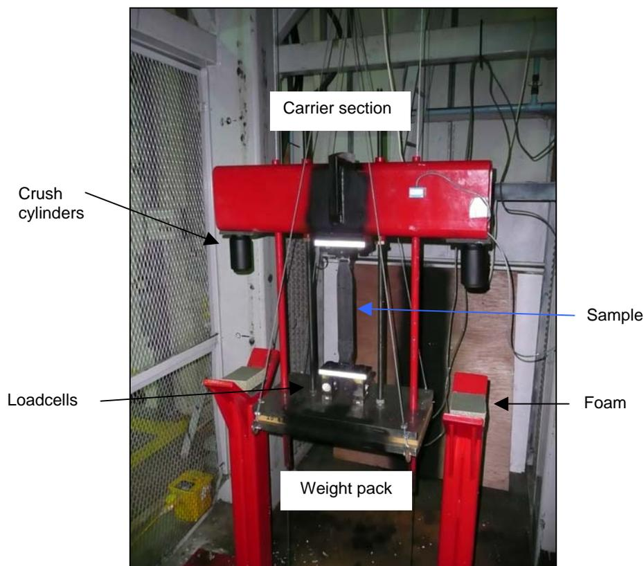
**Figure 17. Photograph of feasibility study test rig**
