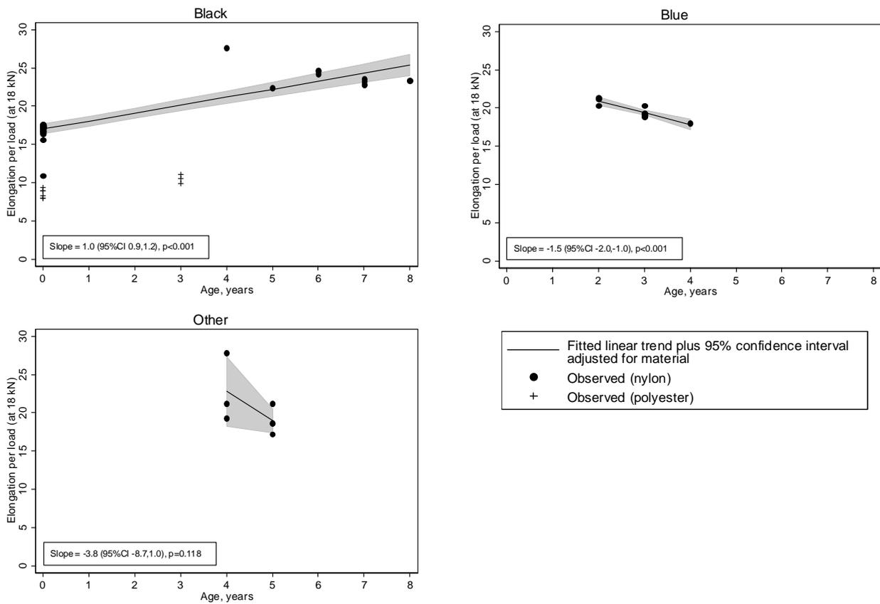
**Figure 38 Fitted linear age trend for elongation per load at 18 kN and strength 3000, by belt colour**
