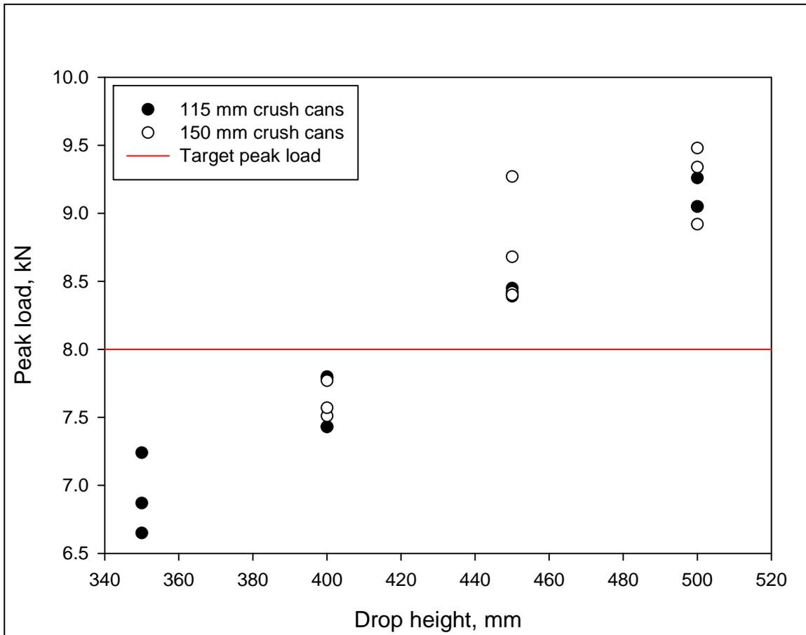
**Figure 28. Graph showing how peak load varies as a function of drop height for a grip separation of 300mm**
