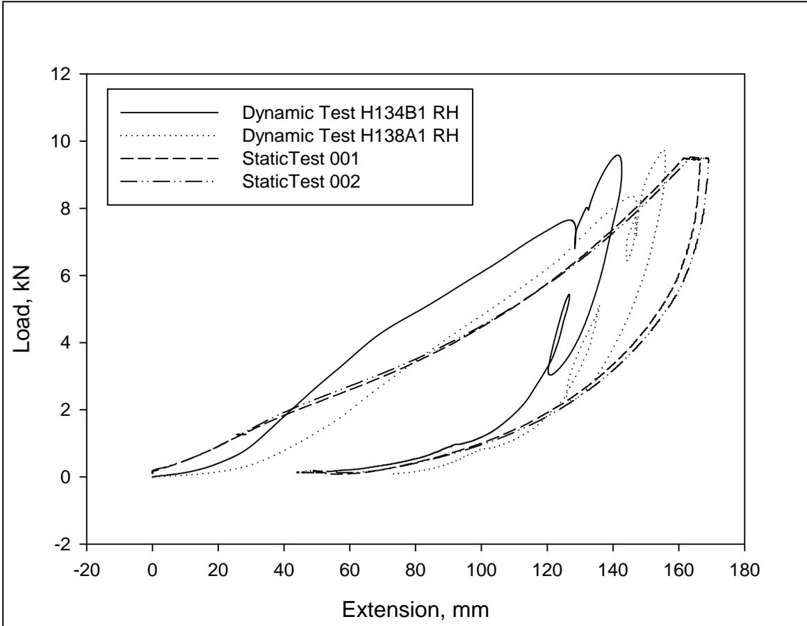
**Figure 12. Comparison of load extension curve for dynamic and static test methods on new nylon belts from manufacturer A.**
