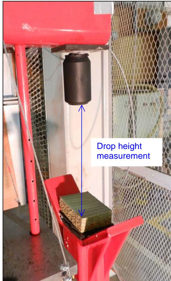
**Figure 26. Measurement of drop height**
