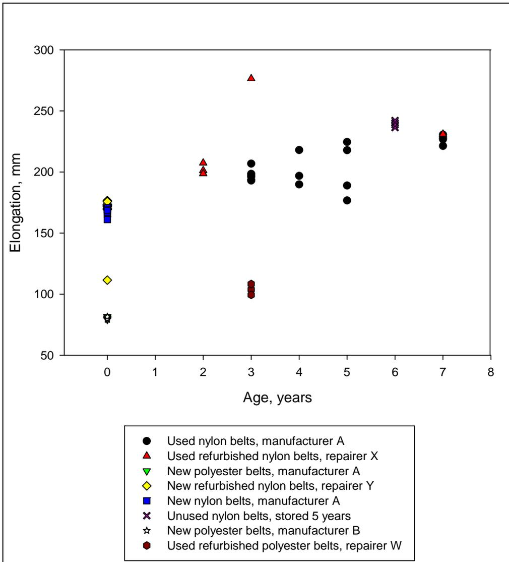
Figure 7. Graph of elongation versus age for 3000lb belts at 18kN static load
