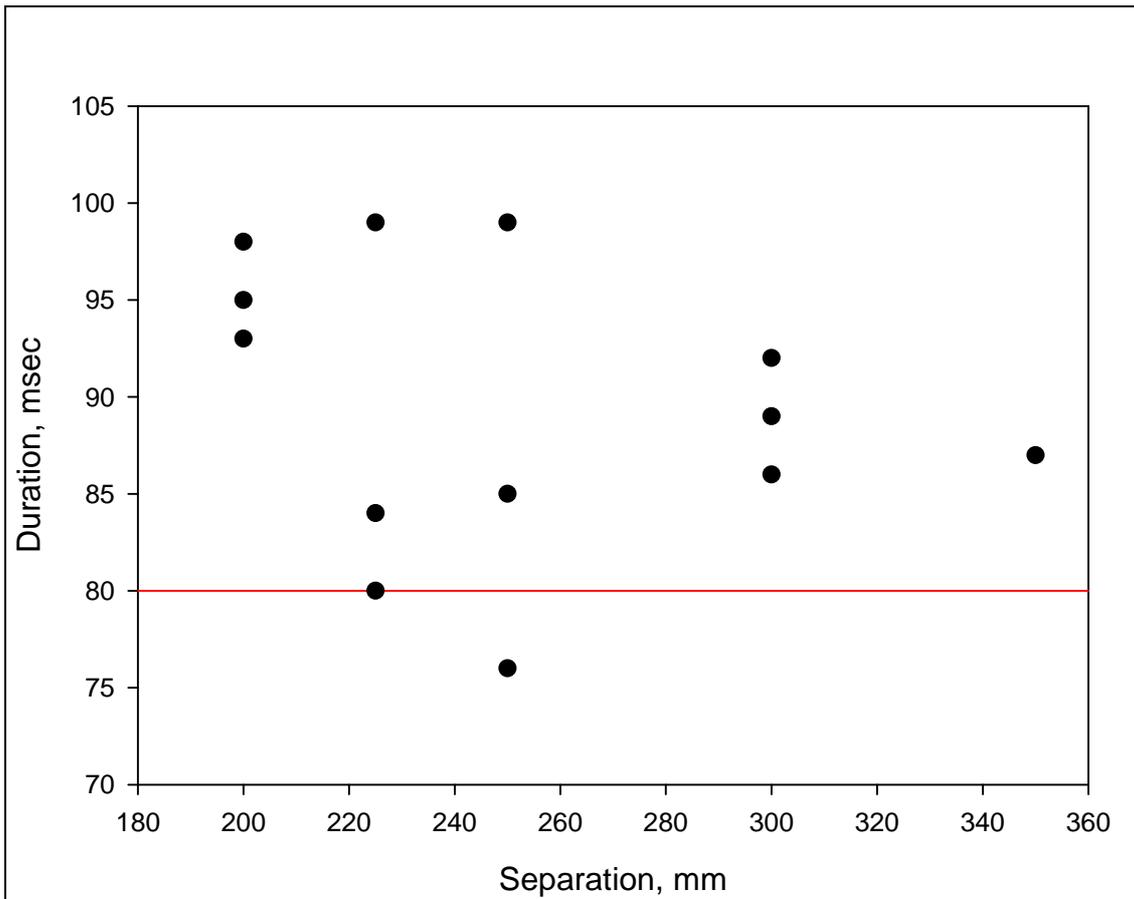
Figure 30 shows how the duration of the load varied according to separation. There appears to be a wide scatter in this data, making it difficult to draw conclusions from it, except that few tests achieved the correct duration.
