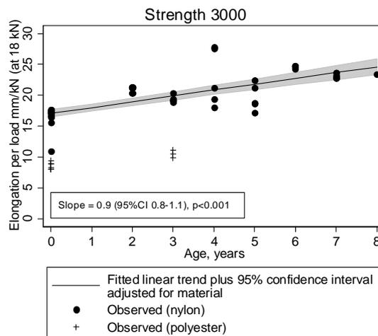
**Figure 36 Fitted linear age trend for elongation per load at 18 kN and strength 3000**
