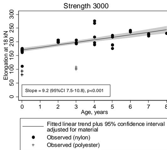
**Figure 33** Fitted linear age trend for elongation at 18 kN and strength 3000
