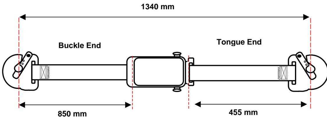
**Figure 1. Dimensions of a 1340mm long belt in its fully extended condition**
