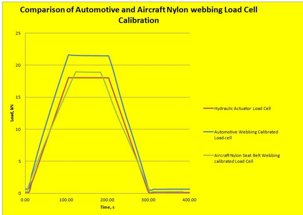
**Figure B.1.3 Comparison of Seat Belt Load Cell loads calibrated with Automotive and aircraft seat belt webbing materials**
