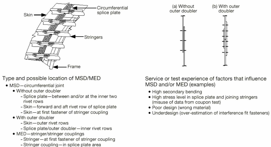
**Figure A2-2 Circumferential Joints and Stringers (MSD/MED)**
