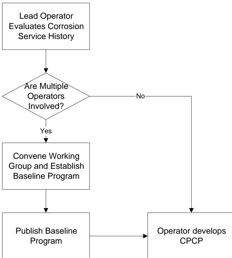
Figure 2-2. Operator Developed Baseline Program
