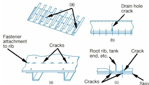
Inherent fail safe and crack stopper characteristics
