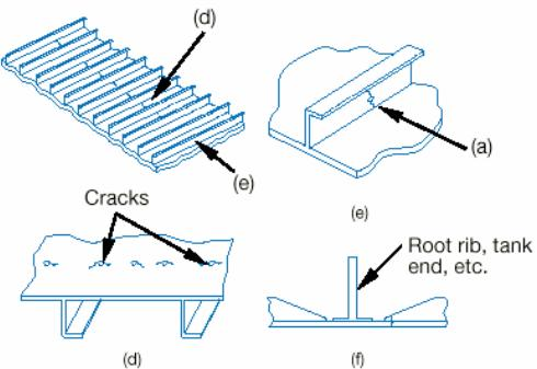
Do not have inherent crack stopper characteristics of riveted skin and stringer construction
