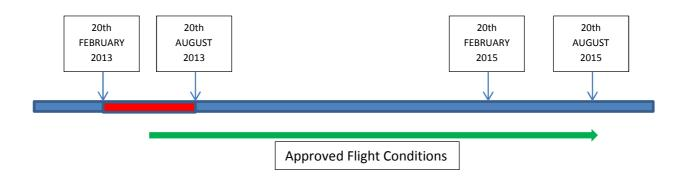
New aircraft S/N could also apply for flight conditions approval from the 20th of August 2013 to the 20th of February 2015 but this will be restricted to aircraft which conform to a type design for which significant progress has been made towards the approval of the Type Certificate or Restricted Type Certificate. The period of validity will be granted until 20th August 2015.
