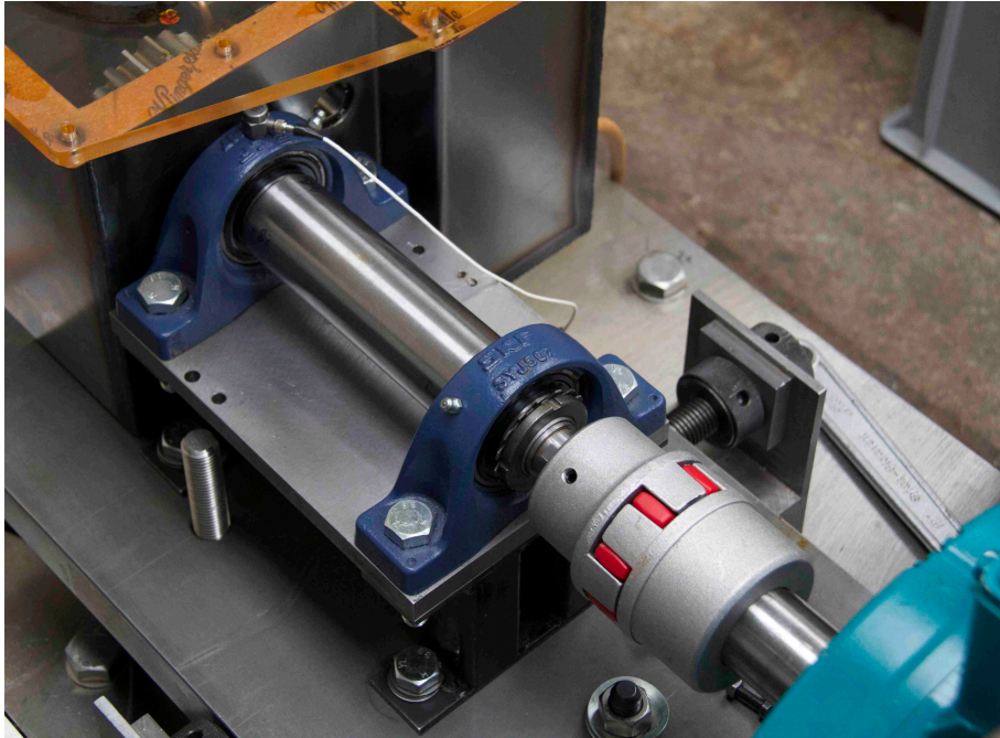
Figure 31. Motor output, coupling and gearbox input shaft
