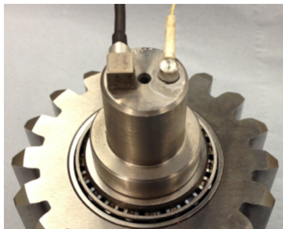
Figure 35. AE sensor and triaxial accelerometer mounted on idler shaft
