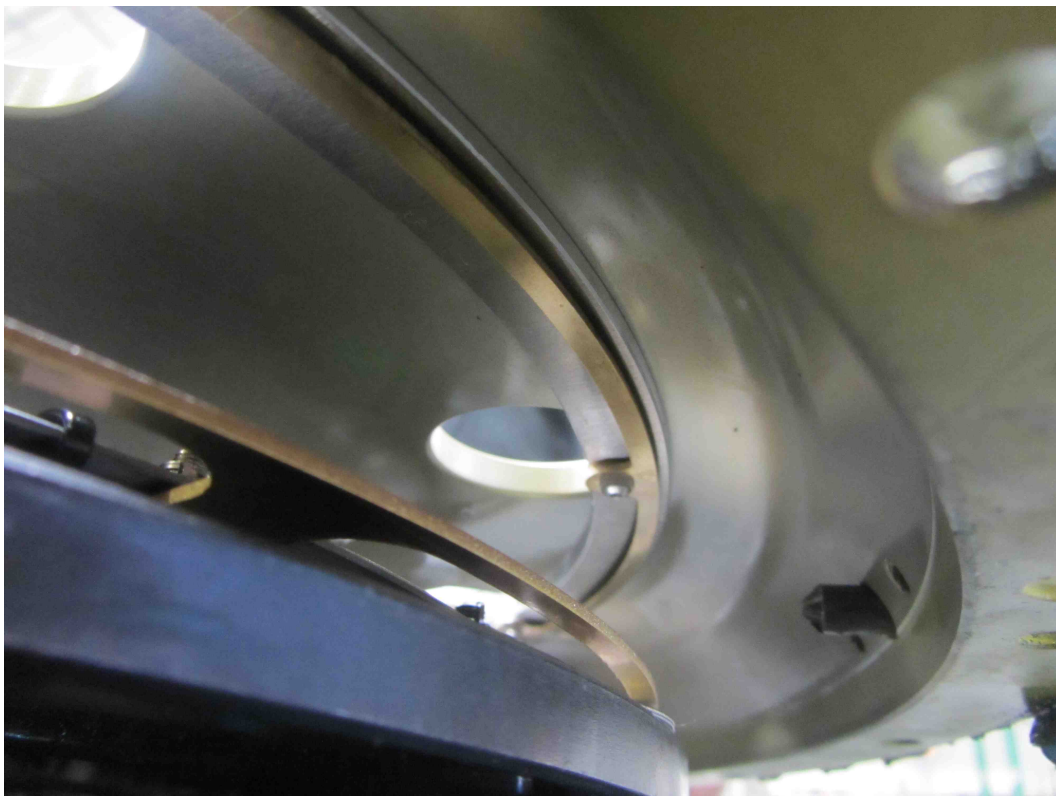
Figure 71. Moving coil (lower) and static coil (upper) before rejoining the two parts
