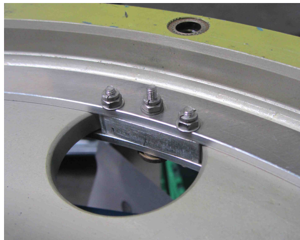
Figure 69. Stationary coil mounted on gearbox top cover
