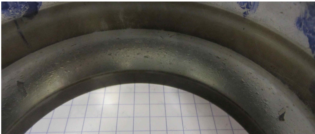
Figure 65. Existing outer race damage
