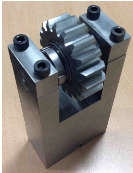
Figure 33. Idler shaft support and idler gear
