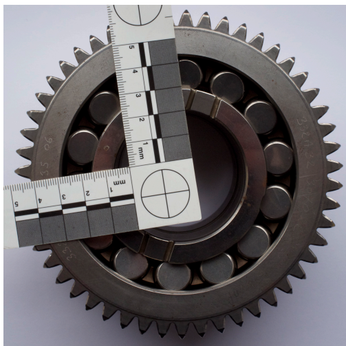
Figure 19. Second stage planetary gear
