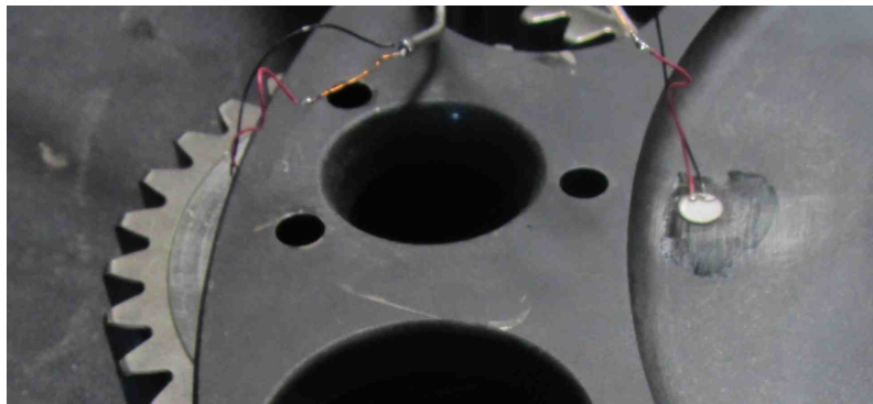
Figure 67. Position of two sensors on planet carrier
