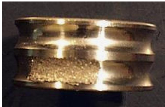
Figure 61. Simulated inner race damage from [185]
