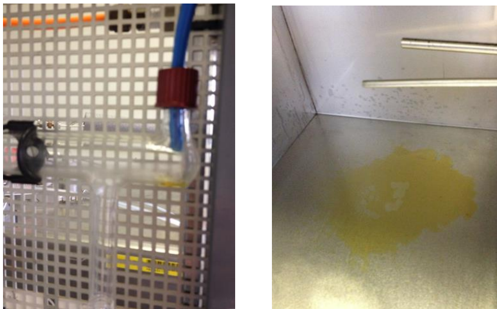
Figure 4.7. Left the condensation of oil nearby the vapour inlet can be seen, while on the right condensation of the oil inside of the emission chamber after a simulation run can be seen.
