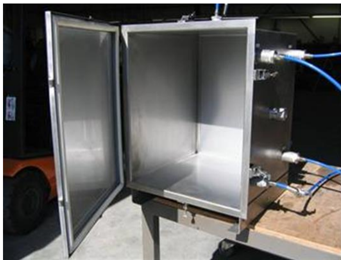
Figure 4.4. The stainless steel emission chamber and its connectors for in- and output of flows.
