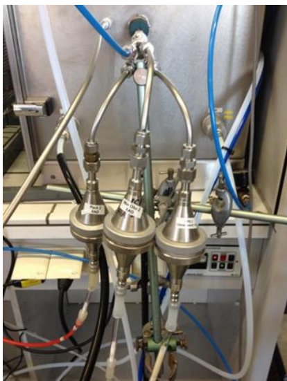
Figure 4.5. The sampling devices for PAHs, mineral oil and OPEs, coupled directly to the emission chamber.
