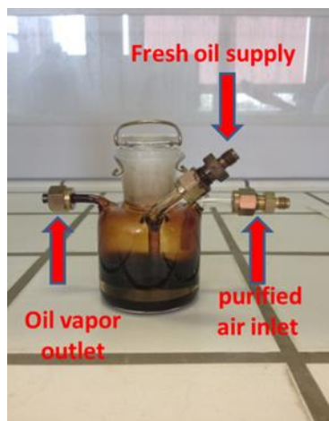
Figure 4.3. The reaction vessel with the three channels for the supply of fresh oil, supply of purified air and to stream the contaminated air out of the vessel to the emission chamber.
