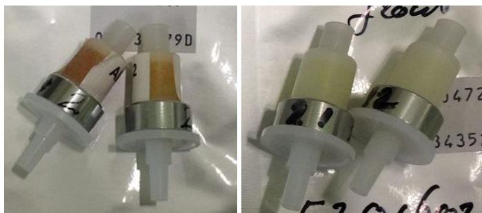
Figure 4.16. Left: DNPH cartridges after sampling oil vapours at 375°C. Right: DNPH cartridges after sampling the blank system at 375°C.
