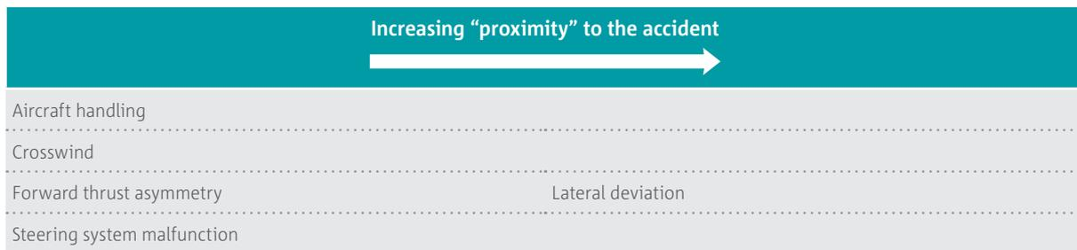
**Aircraft handling:** inappropriate use of aircraft controls (rudder and nose wheel steering) could cause controllability problems. Also, inadvertent actuation of wheel brakes while using the rudder pedals could affect lateral controllability causing lateral deviations (as a form of pilot induced oscillations)
