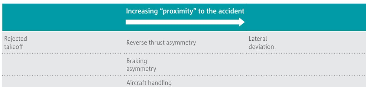
**Rejected takeoff:** in the context of this scenario, the rejected takeoff is the trigger for the chain of events. However in reality it could be the consequence of numerous circumstances which are not relevant for this analysis (tower request, runway incursion by other aircraft, bird strike, or any of the factors listed in the previous accident scenario)
