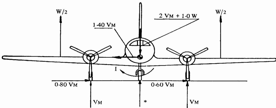
$VM$  = One-half the maximum vertical ground reaction obtained at each main gear in the level landing conditions.
