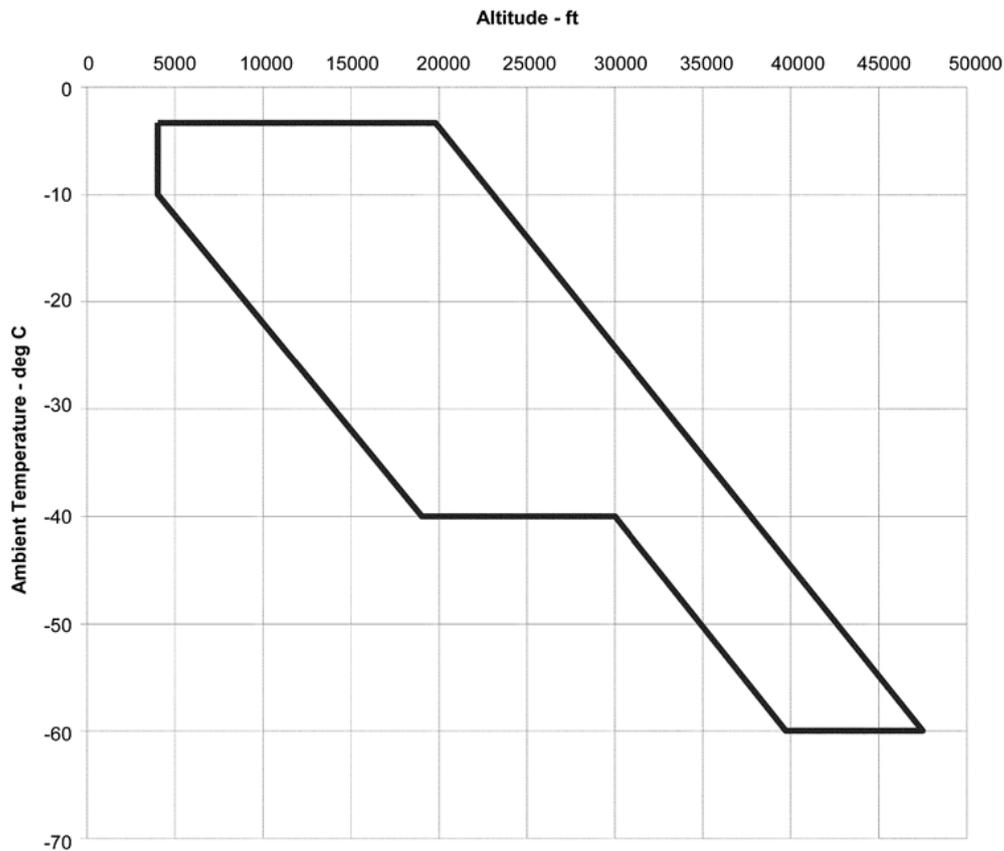
Within the envelope, total water content (TWC) in g/m<sup>3</sup> has been determined based upon the adiabatic lapse defined by the convective rise of 90 % relative humidity air from sea level to higher altitudes and scaled by a factor of 0.65 to a standard cloud length of 32.2 km (17.4 nautical miles). Figure 2 displays TWC for this distance over a range of ambient temperature within the boundaries of the ice crystal envelope specified in Figure 1.
