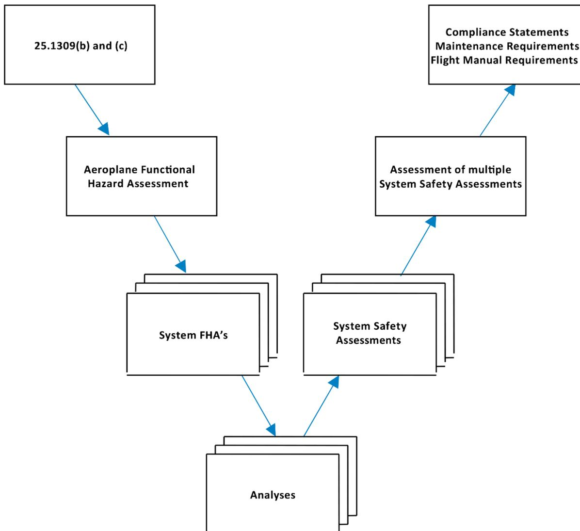
Figure A2-2: Depth of Analysis Flowchart
