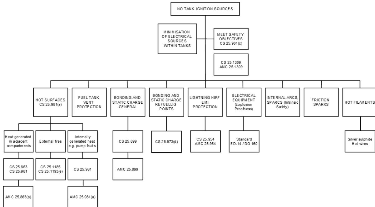
Therefore the focus of this evaluation of the aircraft fuel system should be to identify and address potential sources of ignition within fuel tanks, which may not previously have been considered to be unsafe features.
