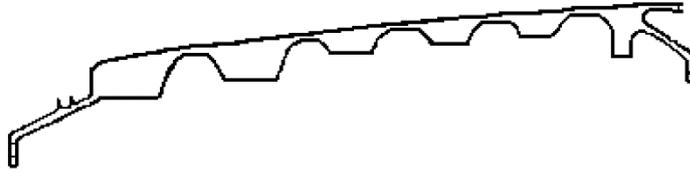
**4.a - Ring Disk Drum Rotor Cross Section**
