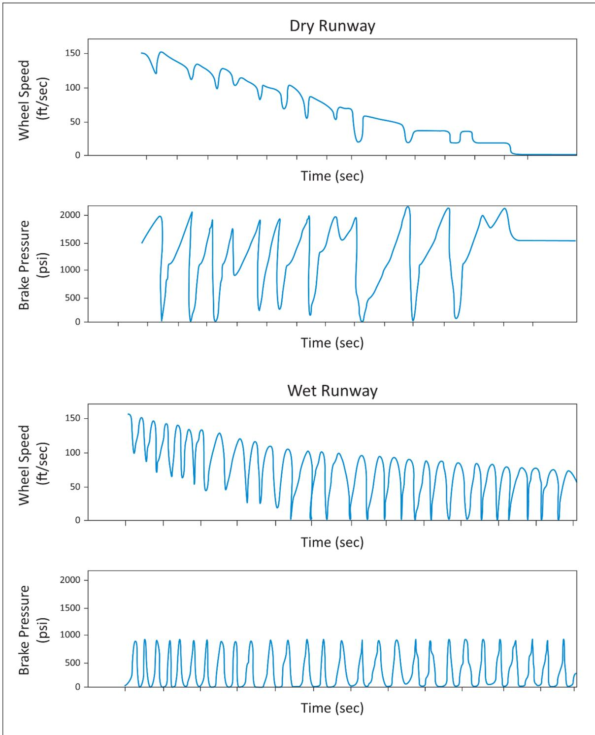
**FIGURE 2. ANTI-SKID SYSTEM RESPONSE CHARACTERISTICS Quasi-Modulating System**
