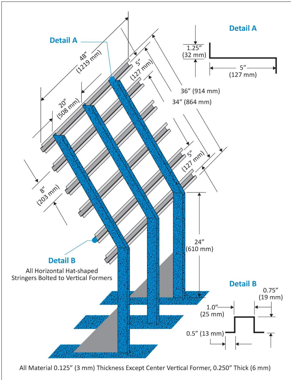
**Figure 1 – Burnthrough Test Apparatus Specimen Holder**
