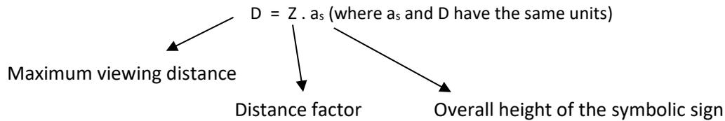
The maximum viewing distance "D" can be calculated from the overall height of the symbolic sign (as) by using the appropriate distance factor Z obtained from Table 1 below.
