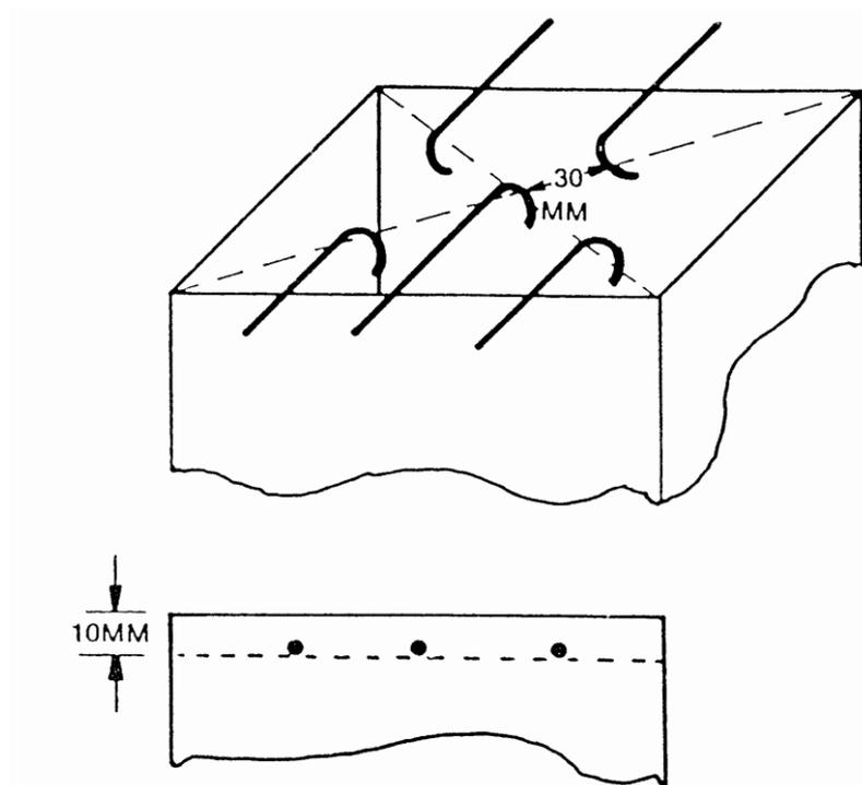
**FIGURE 5. THERMOCOUPLE POSITION**
