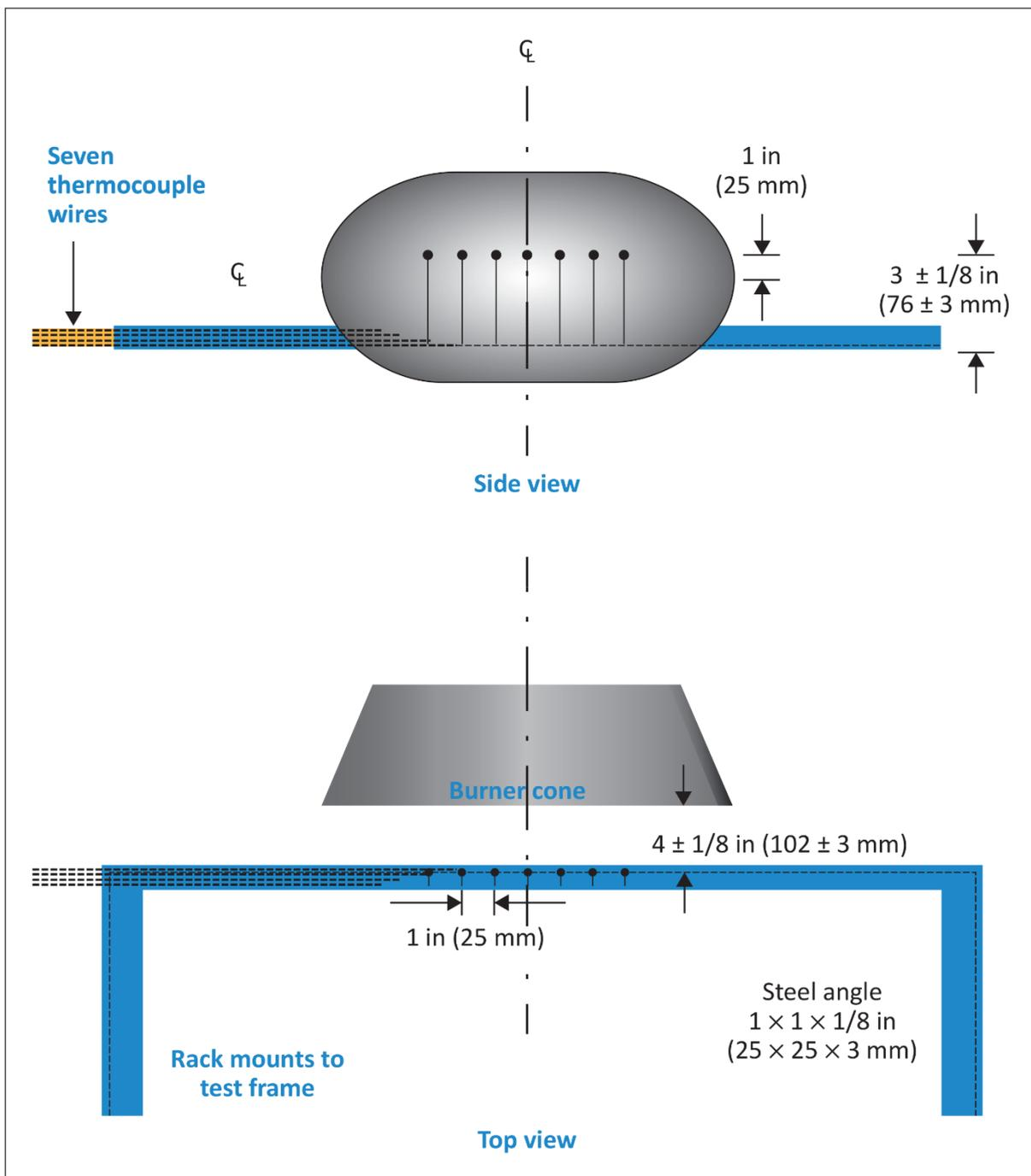
Figure 5 – Thermocouple Rake Position Relative to Burner Cone
