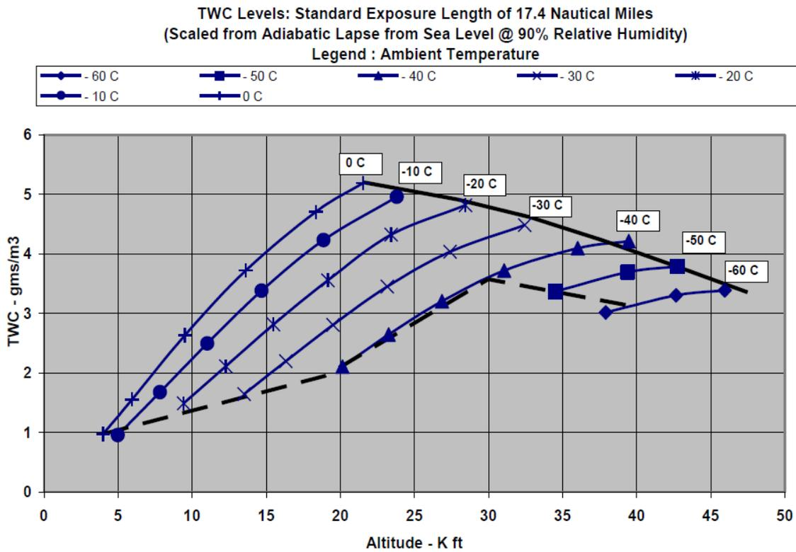
Ice crystal size median mass dimension (MMD) range is 50–200 microns (equivalent spherical size) based upon measurements near convective storm cores. The TWC can be treated as completely glaciated (ice crystal) except as noted in the Table 1.
