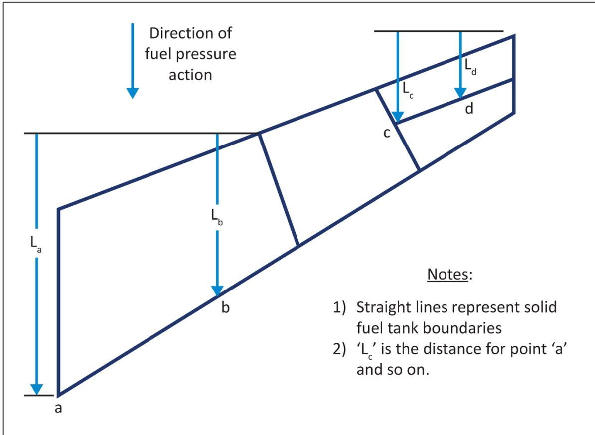
**Figure 4 – Example of Distances for Fuel Outboard Acting Design Pressure Calculations**
