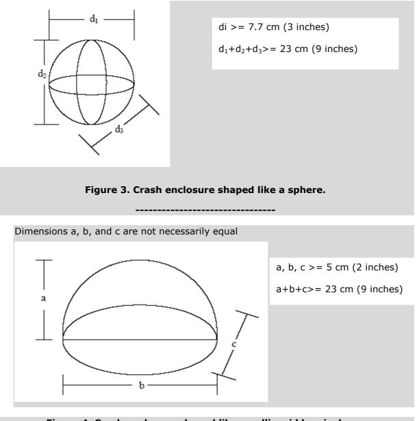
Figure 4. Crash enclosure shaped like an ellipsoid hemisphere.
