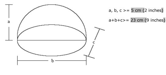
Figure 4. Crash enclosure shaped like an ellipsoid hemisphere.
