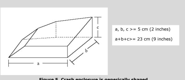
Figure 5. Crash enclosure is generically shaped.
