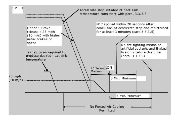
Figure 3-1 - Taxi, Accelerate-Stop, Park Test Sequence
