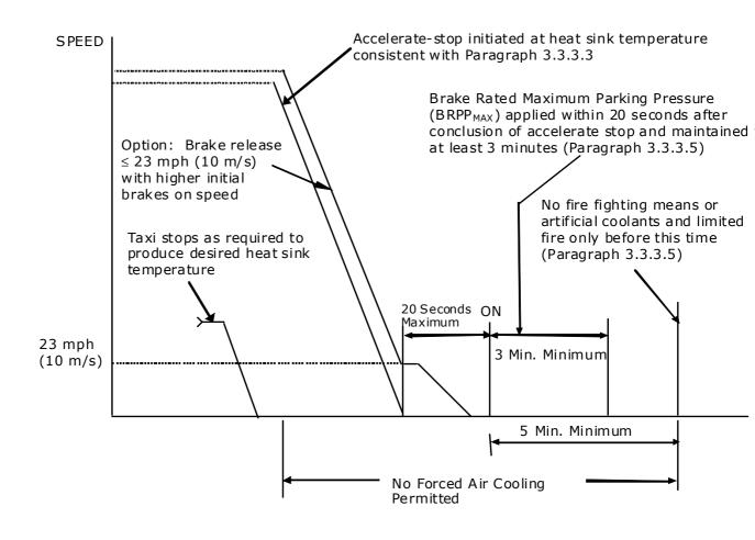
Figure 3-1. Taxi, Accelerate-Stop, Park Test Sequence
