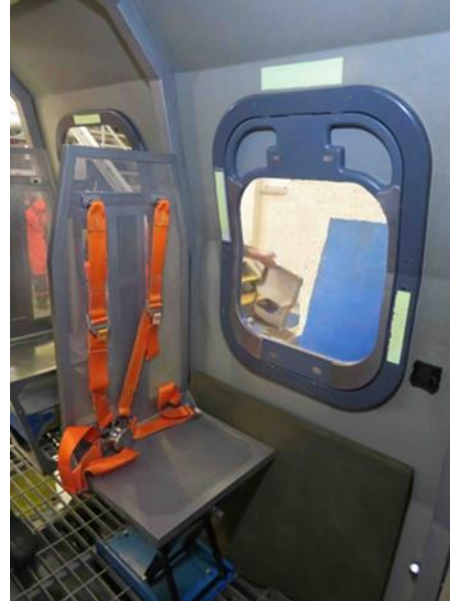
Simulated Type IV push-out exit in HUET
