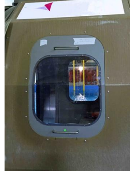
Simulated Type IV push-out exit in HUET
