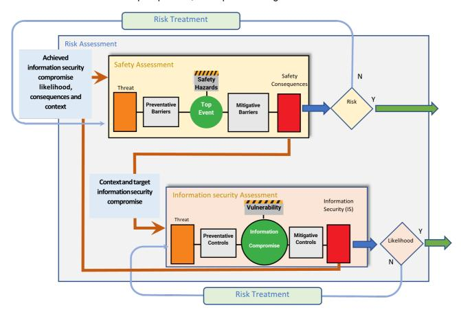
Figure 1 — Bow-tie representation of management of aviation safety risks posed by information security (IS) threats
