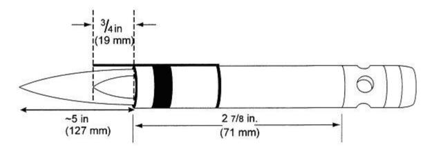
Figure 6 - Propane Pilot Burner
