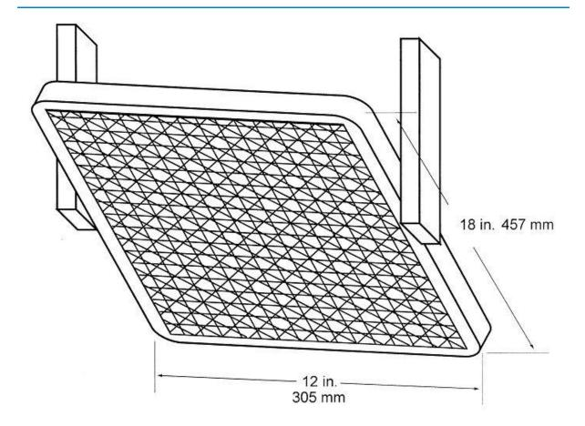
Figure 3b – Air Propane Radiant Panel
