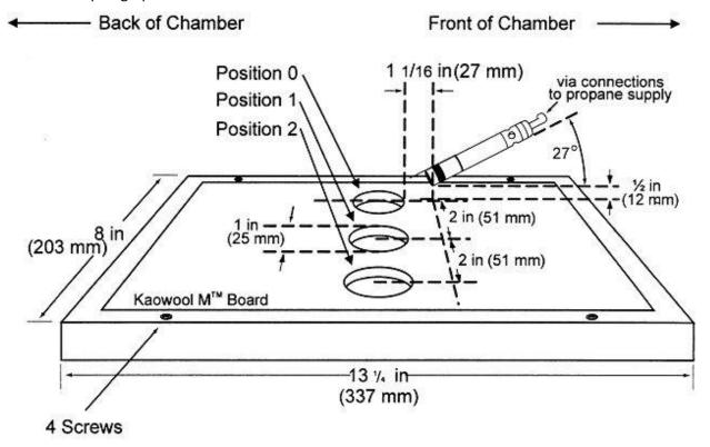
Figure 7 - Calorimeter Holding Frame
