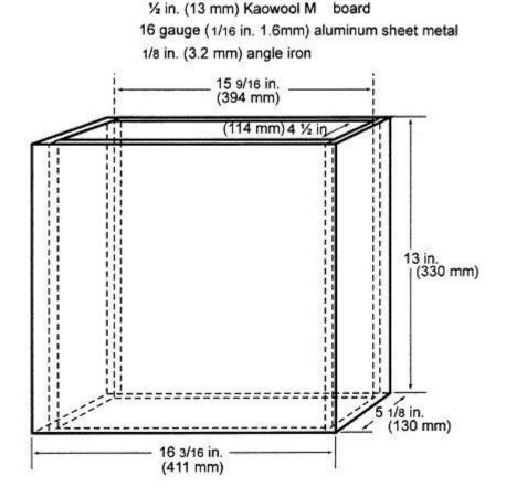
Figure 2 - Internal Chimney
