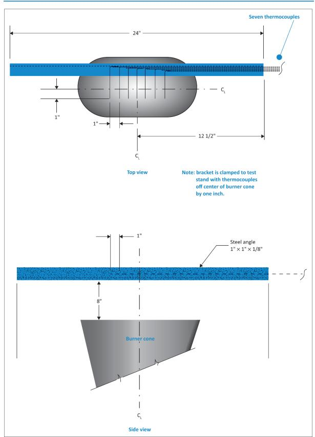
FIGURE 3 THERMOCOUPLE RAKE BRACKET
