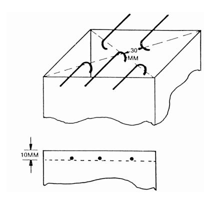
FIGURE 5. THERMOCOUPLE POSITION
