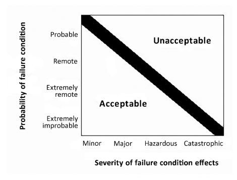
b. The safety objectives associated with Failure Conditions are described in Figure 2.
