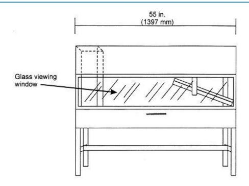
Figure 1 - Radiant Panel Test Chamber
