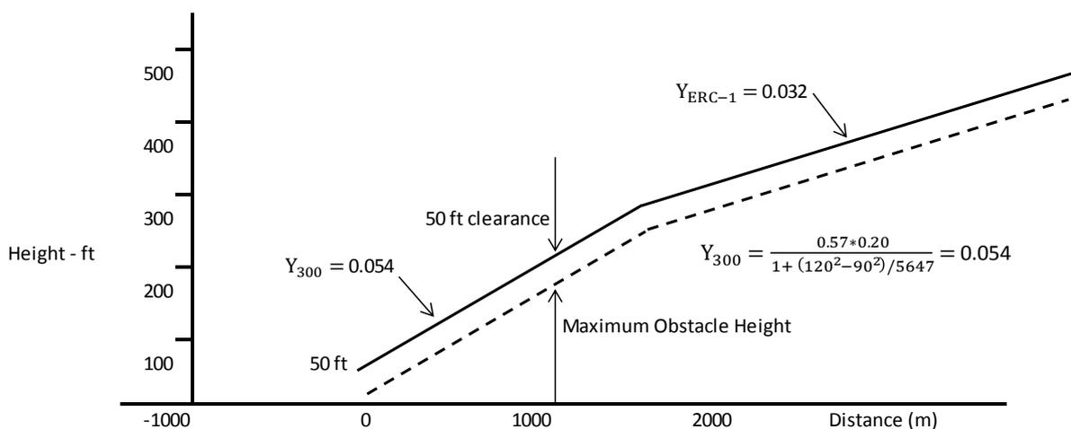
(2) Assumed engine failure height 200 ft
