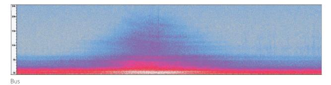
There are elements of tonality at frequencies where they might be expected, such as low frequencies for the bus. There is generally a clear tonal component at around 3kHz for most drones/air taxis, which would correspond to frequencies where humans are most sensitive. However, the tonality is much more distinct with the air taxis than with the drones, which may be a factor in their higher annoyance rating.
