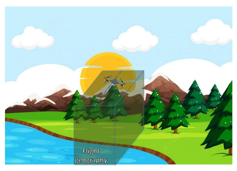
**Flight geography**: where the drone should fly in normal conditions
