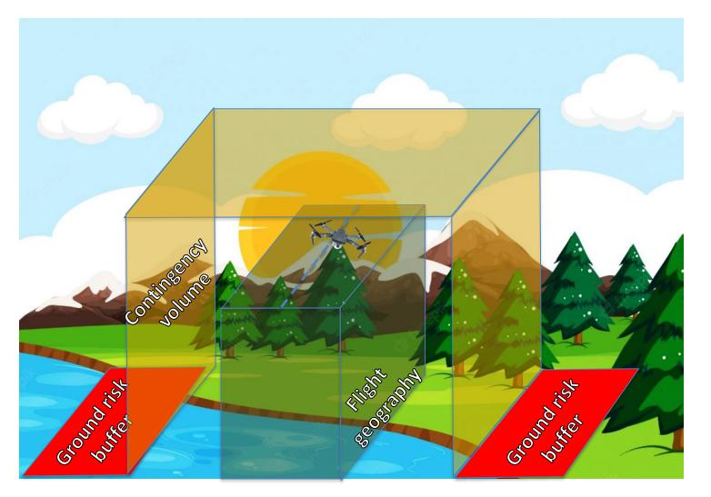
Ground risk buffer: If an operation loses control in a way that the UA exits the operational volume, it shall be contained to end its flight inside the ground risk buffer
