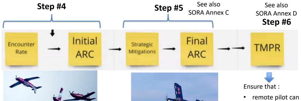
Calculate the probability of encountering manned aircraft in the **EASA**area of operation
