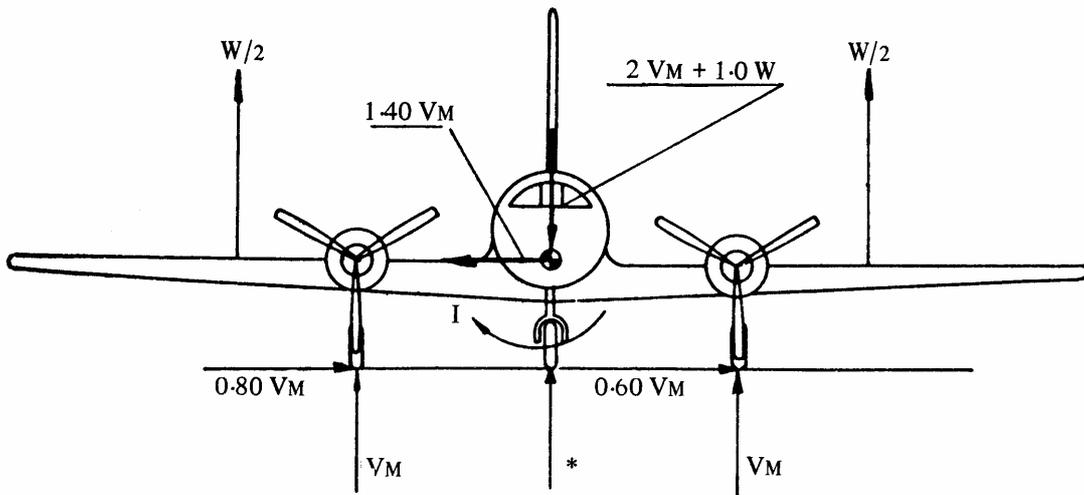
$VM$  = One-half the maximum vertical ground reaction obtained at each main gear in the level landing conditions.
