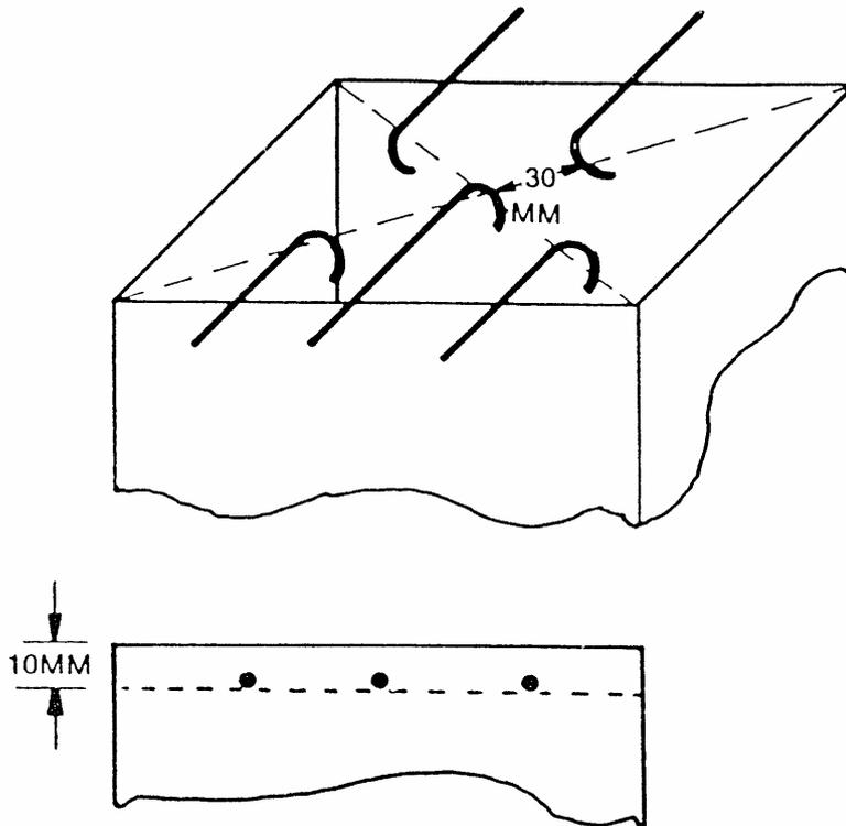
FIGURE 5. THERMOCOUPLE POSITION
