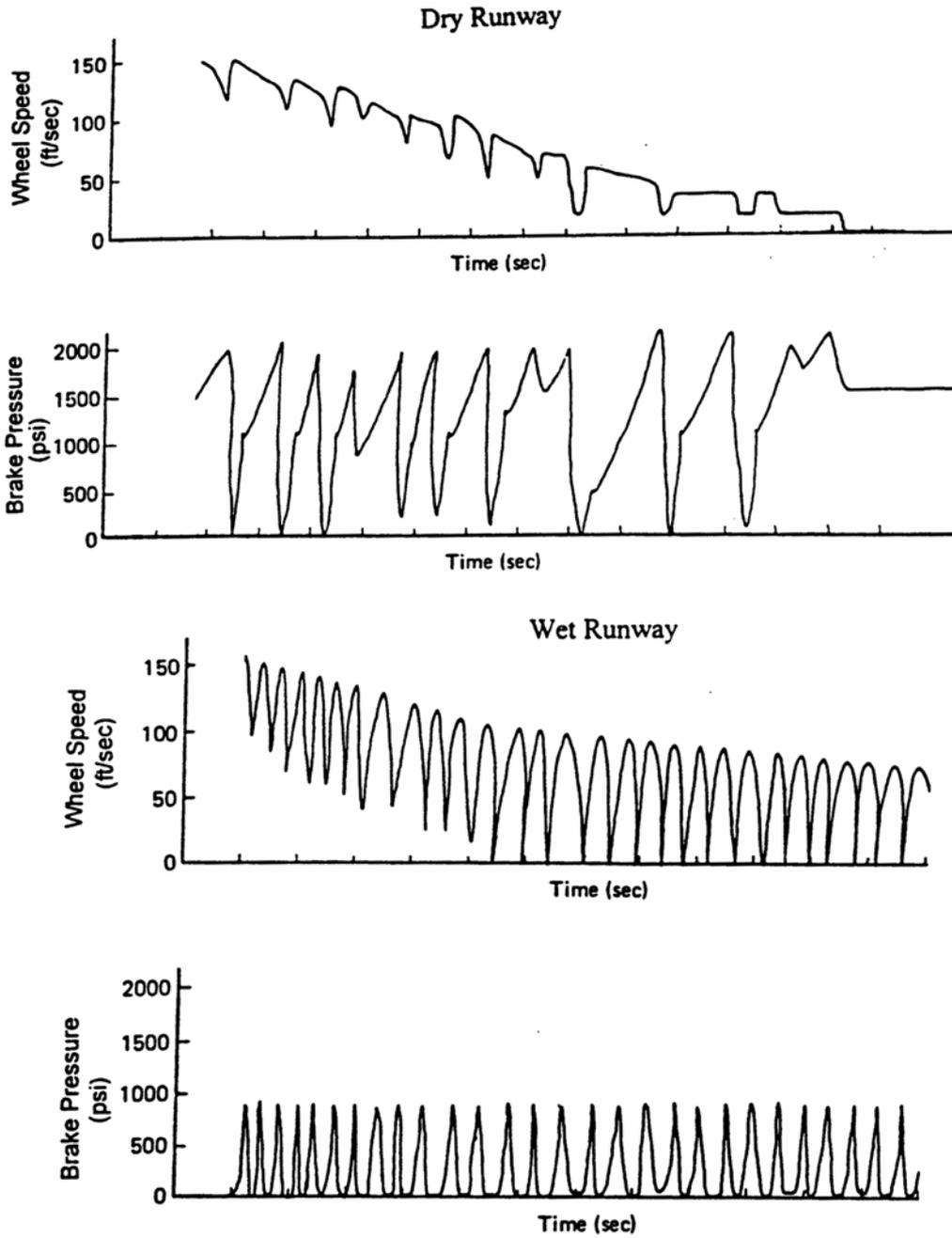
FIGURE 2. ANTI-SKID SYSTEM RESPONSE CHARACTERISTICS
