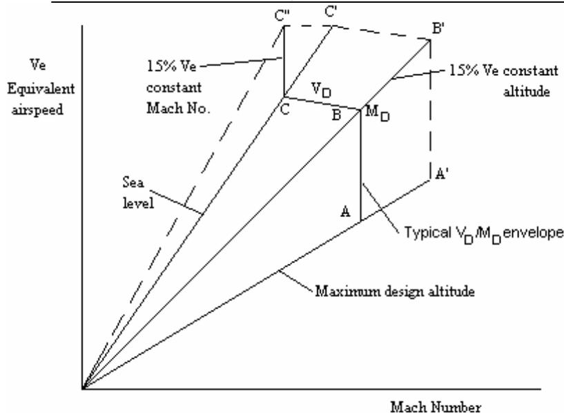
FIGURE 1B MINIMUM FAIL-SAFE CLEARANCE ENVELOPE
