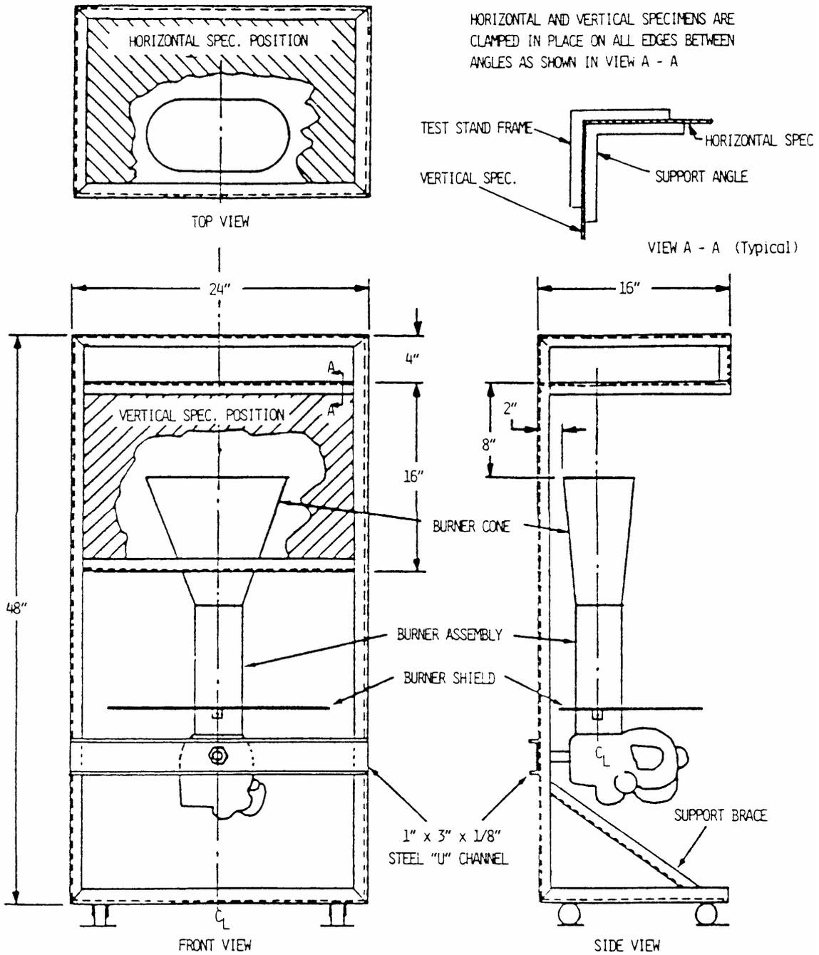
TEST STAND IS CONSTRUCTED WITH 1" x 1" x 1/8" STEEL ANGLES, ALL JOINTS WELDED
