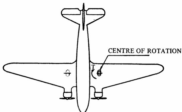
VN AND VM ARE STATIC GROUND REACTIONS. FOR TAIL-WHEEL TYPE THE AEROPLANE IS IN THE THREE POINT ATTITUDE. PIVOTING IS ASSESSED TO TAKE PLACE ABOUT ONE MAIN LANDING GEAR UNIT.
