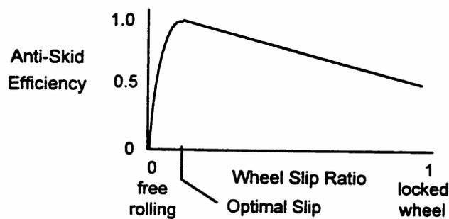
**FIGURE 5. ANTI-SKID EFFICIENCY – WHEEL SLIP RELATIONSHIP**
