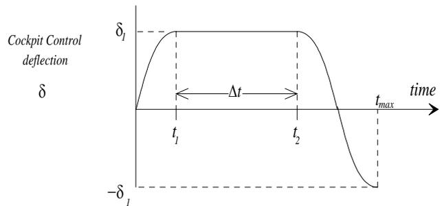
(iv) In cases where the cockpit pitch control motion may be affected by inputs from systems (for example, by a stick pusher that can operate at high load factor as well as at 1g) then the effects of those systems must be taken into account.
