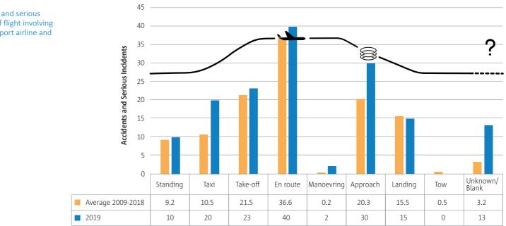
**Figure 10** Accidents and serious incidents by phase of flight involving commercial air transport airline and air-taxi aeroplanes
