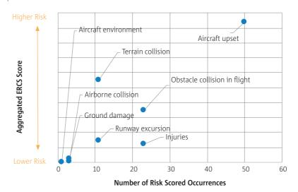
From the data, it can be observed that the aircraft upset accident scenario is the top key risk area, both in terms of the number of occurrences and the aggregated risk. Terrain collisions and obstacle collisions in flight are the other main key risk areas of the specialised operations helicopters domain.
