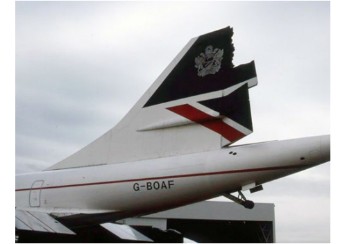
G-BOAF – failed rudder
