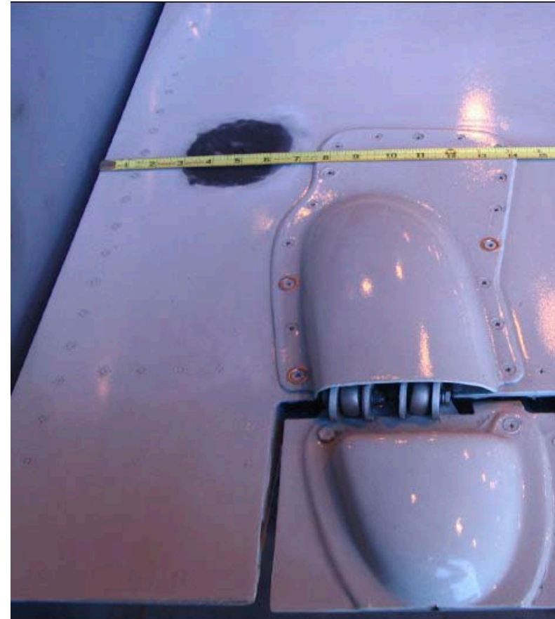
Elevator skin puncture in critical area
