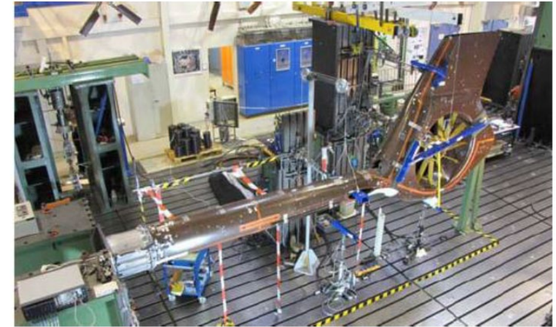
Fig.11: Static test article of tail boom structure *
