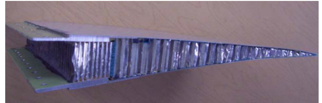
Aluminum core edge with inadequate close-out
