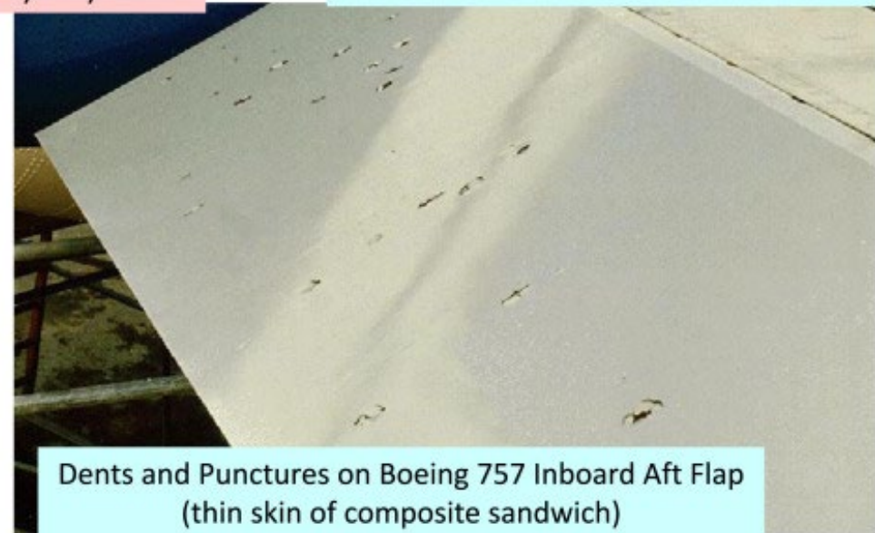
Example of Hail Damage from 1999 Sydney Storm
