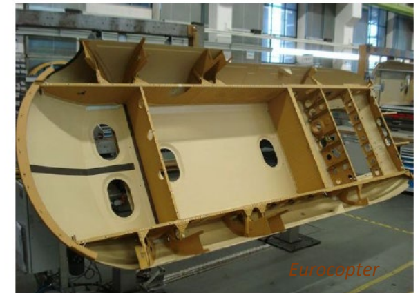
Fig.1.b: EC135 Sub floor group structure
