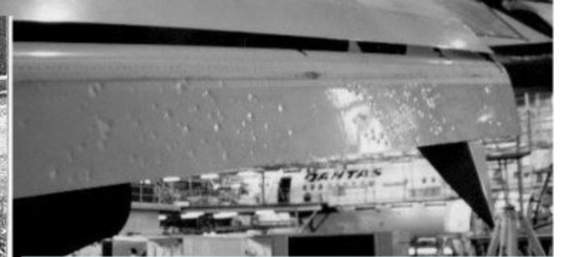
Dents on Boeing 777 Aft Flap (thin skin metal bonded sandwich)
