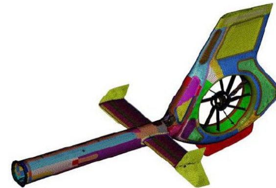
Fig.11: Static test article of tail boom structure *
