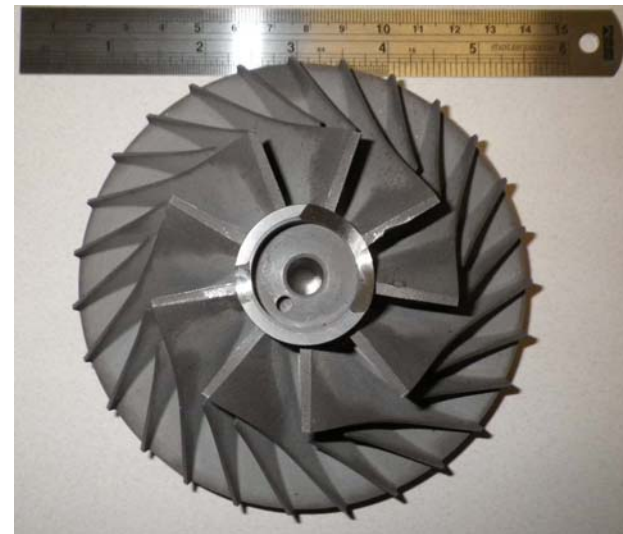
Blower Impeller (70000 rpm)
