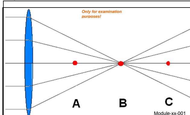
*In the diagram above, parallel light rays pass through a convex lens and converge to a focus. They can be made parallel again by placing a:*
