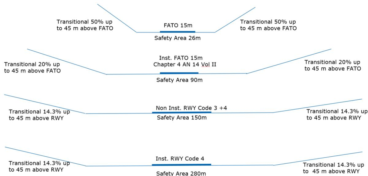
*Instrument FATO:* The obstacle protection, lighting and minimum dimensions of an instrument heliport should be sufficient to avoid any increase in the operating minima. No increase in the operating minima should apply.
