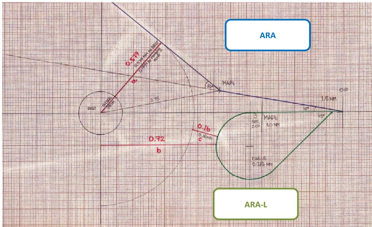
On the illustration above, both ARA and ARA-L are presented. ARA will provide a 0.579-NM (line a) clearance at its closest; if the ranging error of  $\pm 250$  NM/0.1350 NM is subtracted, the clearance is 0.444 NM. (The ranging error has been drawn around destination point for simplicity.) On the other hand, ARA-L will provide approximately a 0.720-NM (line b) clearance to 'land' (or approx. 0.585 NM considering the ranging error).
