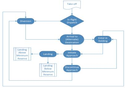
The pilot-in-command shall continually ensure that the amount of usable fuel remaining on board is not less than the fuel required to proceed to an aerodrome where a safe landing can be made with the planned final reserve fuel remaining upon landing.
