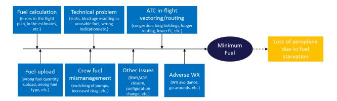
Figure 2 — Theoretical causes of a minimum-fuel scenario
