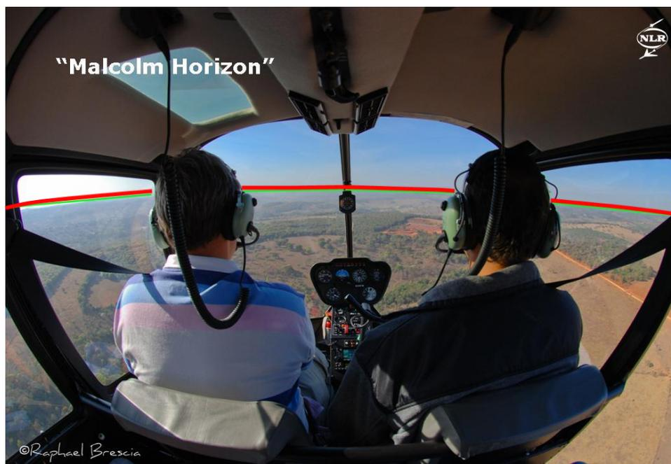
*Figure 4 Extended horizon line or Malcolm Horizon (MH) concept*
