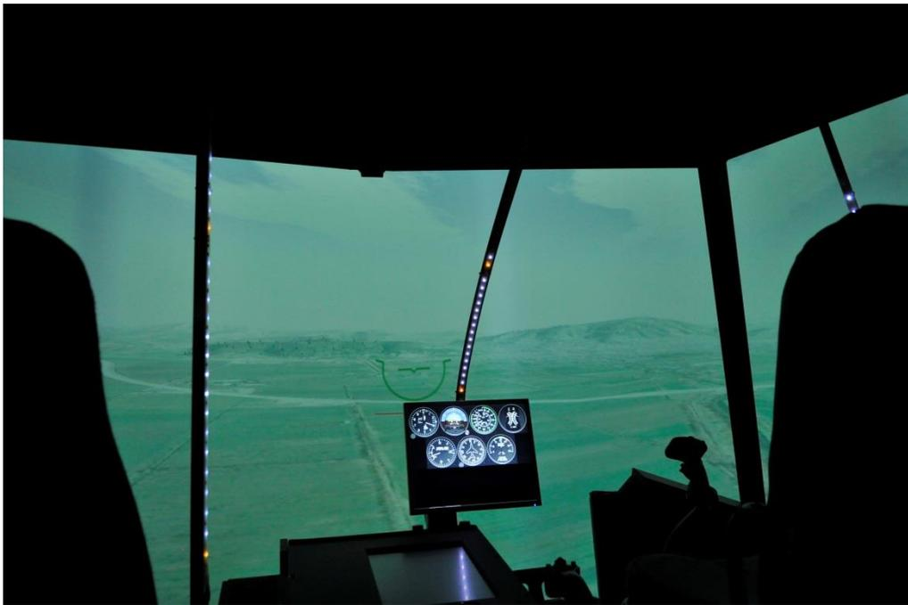
*Figure 15 LED concept with amber-colored upward-traveling lights*
