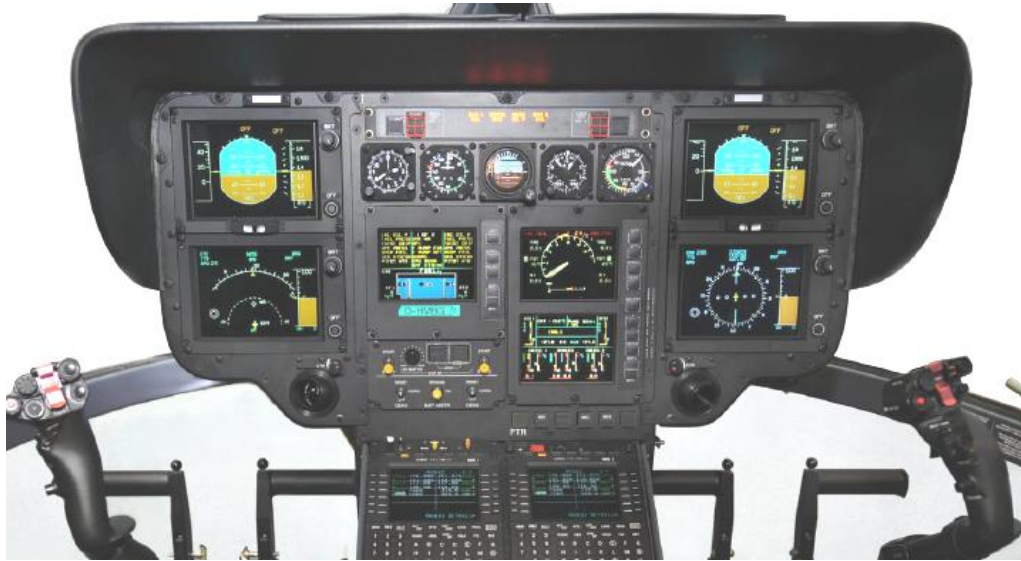
(EC145 / BK117 C-2) digital CPDS cockpit with FCDS flight instrumentation
