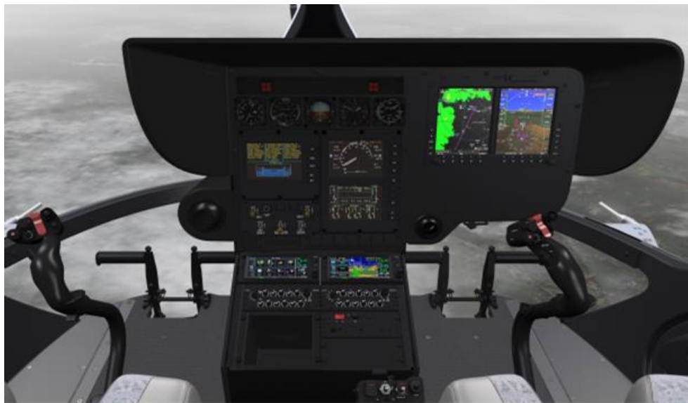
(EC145 / BK117 C-2e) digital CPDS cockpit with Garmin G500H flight instrumentation
