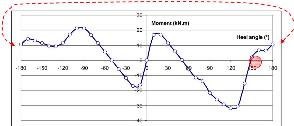
Figure 9: AS355 - Stability curves with one 1500L upper float
