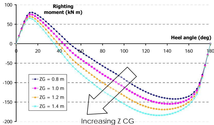
**Figure 12: EC225 - Influence of the CG's height on the helicopter stability**
