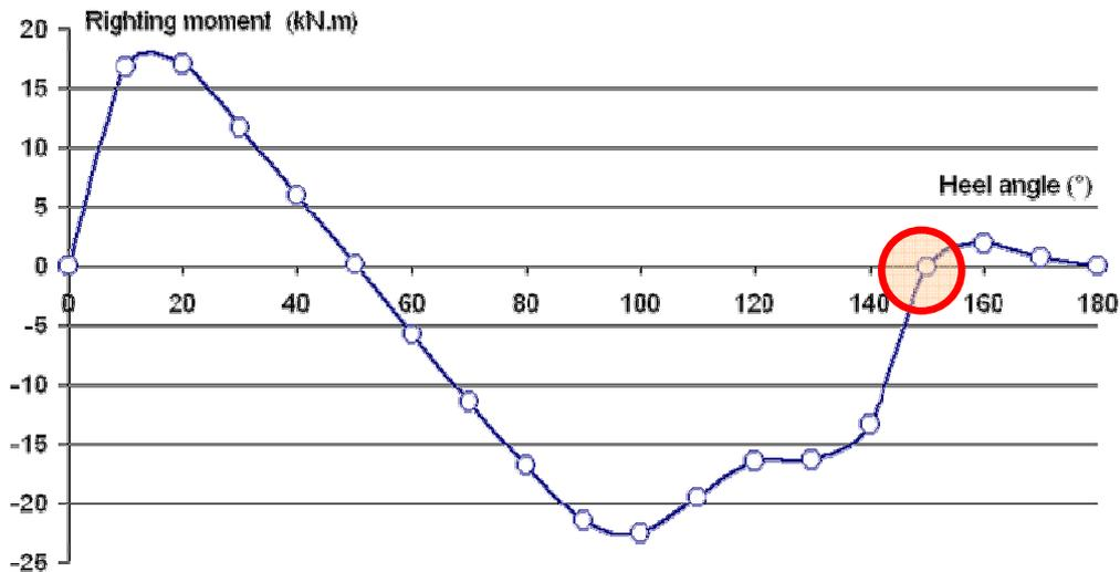
Figure 8: AS355 – Stability curve with 2x1000L upper floats
