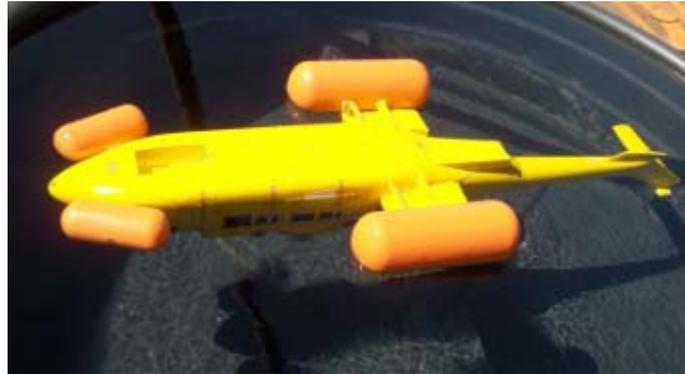
**Figure 16: EC225 - Fully inverted position (C1)**
