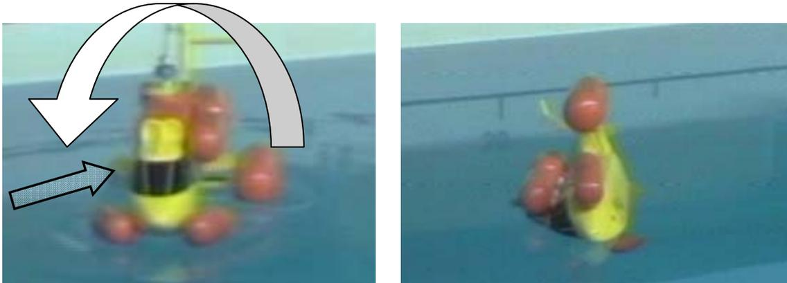
Figure 21: EC225 – Water impact - Config C5 – Rear port side float removed.
