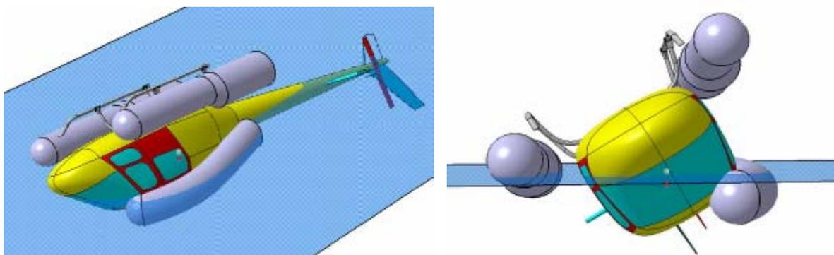
Figure 10: AS355 – Inclined position with one 1500L upper float
