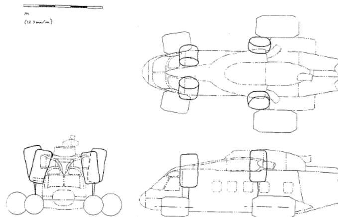
Figure 3: Tethered inflatable floatation units
