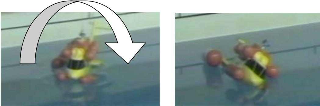
Figure 23: EC225 – Water impact - Config C6 – Rear starboard float removed.
