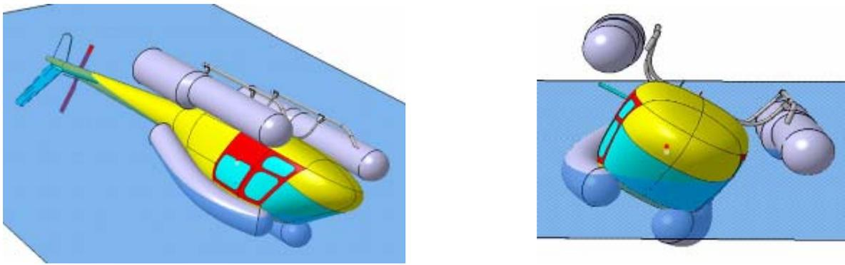
Figure 7: AS355 – Inclined position with 2x1000L upper floats
