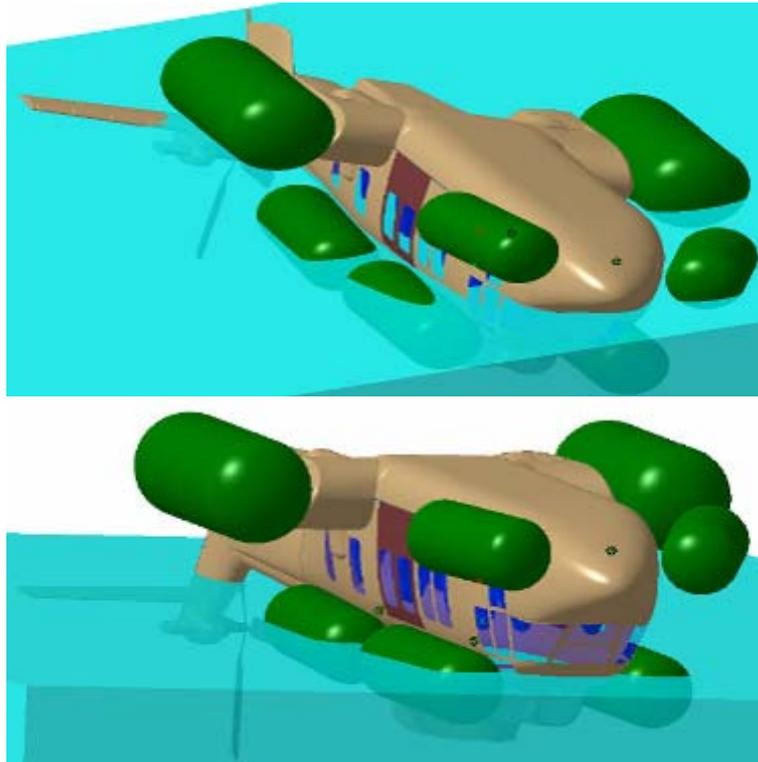
Figure 17: EC225 – Equilibrium positions for configuration 3. Up: AV1. Down: AV3
