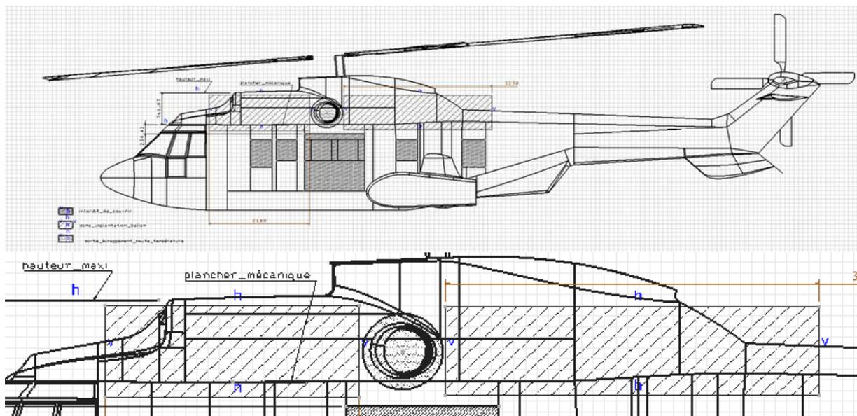
Figure 25: Lateral views of the EC225 with the possible locations of additional floats
