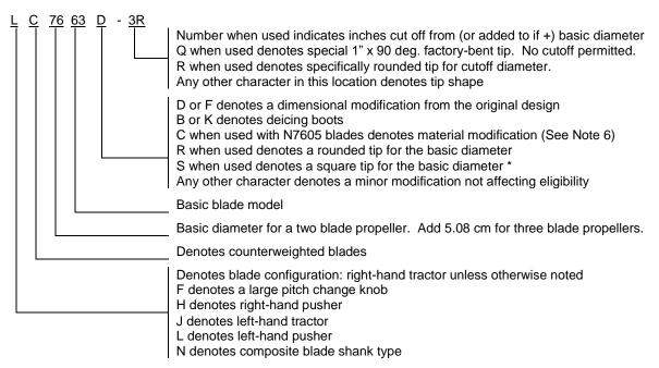
Blades may incorporate either round or square tips, yet may not be marked with an "R" or "S" in their model designation. This character is used to distinguish between two or more tip shapes available at the same diameter. Certain blades use "S" to denote shot peening of the exterior surface. (See Note 6)
