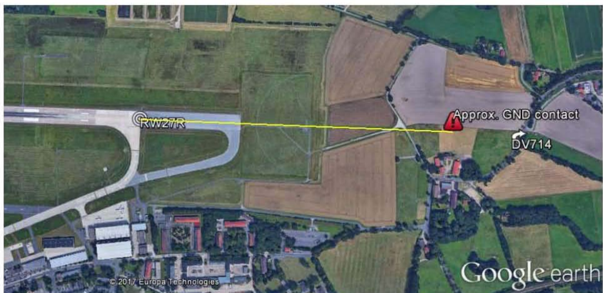
Figure 3-10: The lowered threshold height leads to a potential ground contact approximately 0.5 NM (yellow line) before the threshold, shortly after passing the missed approach point DV714.
