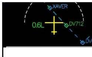
Figure 6-5: Lateral deviation after GNSS spoofing during approach.
