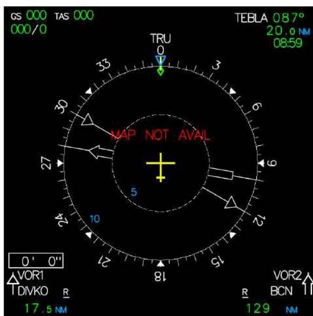
Figure 3-9: Navigation display (ND) showing the MAP NOT AVAIL flag.
