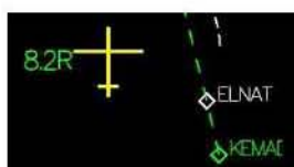
Figure 6-4: Lateral deviation after GNSS spoofing en-route.
