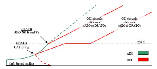
Otherwise, and if scheduled in the AFM, the AEO distance to 50 ft ( $V_{50}$ ) — determined in accordance with CS/JAR 29.63 — can be used (see Figure 7). Where this distance is used, it will be necessary to ensure that the  $V_{50}$  climb out speed is associated with a speed and mass for which OEI climb data are available so that, from  $V_{50}$ , the OEI flight path can be constructed.
