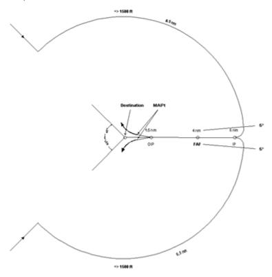
**Figure 2**Base turn procedure — direct approach
