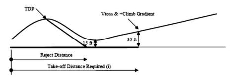
The operator only has to establish that the distances required are within the distance available (take-off distance and reject distance). The original definition of TODRH meets this case exactly.
