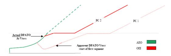
The apparent DPATO is for planning purposes only in the case where AEO data are not available to construct the take-off flight path. The actual OEI flight path will provide better obstacle clearance than the apparent one (used to demonstrate the minimum requirement) — as seen from the firm and dashed lines in the above figure.
