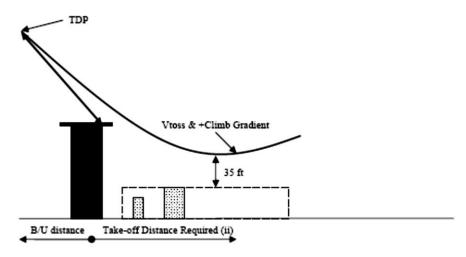
The main difference is that drop down below the level of the take-off surface is permitted. In the drop down phase, the Category A procedure ensures deck-edge clearance but, once clear of the deck-edge, the 35 ft clearance from obstacles relies upon the calculation of drop down. Subparagraph (b) of AMC1 CAT.POL.H.205(b)(4) is applied.
