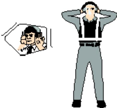
**27. Establish communication via interphone (technical/servicing communication signal)**
