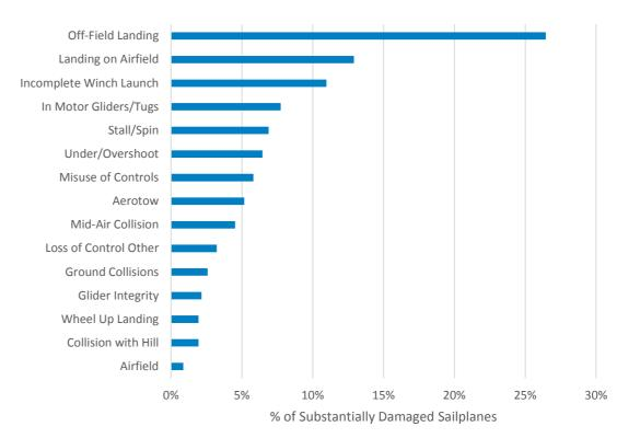
**Figure 68.** Percentage Of Substantially Damaged Or Destroyed Sailplanes By Safety Issue, 2014-2018 The main Safety Issues are:
