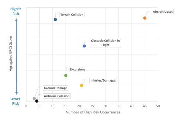
**Figure 49.** Comparison Of Number Of Occurrences And Aggregated ERCS Score Per Key Risk Area, 2014-2018 The main key risk areas identified and prioritised using the ERCS risk score methodology are Aircraft Upset, Terrain Collision and Obstacle Collision in Flight. One single occurrence can be connected to more than one key risk area.
