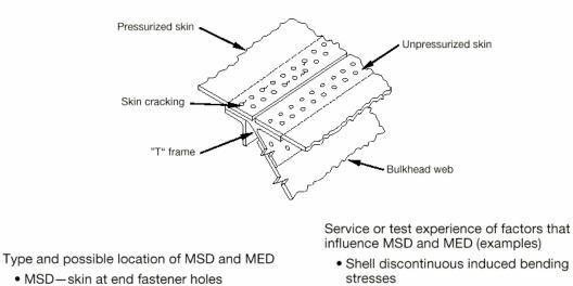
High load transfer at fastener
