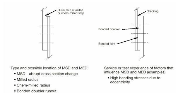
Figure A2-2 Circumferential Joints and Stringers (MSD/MED)
