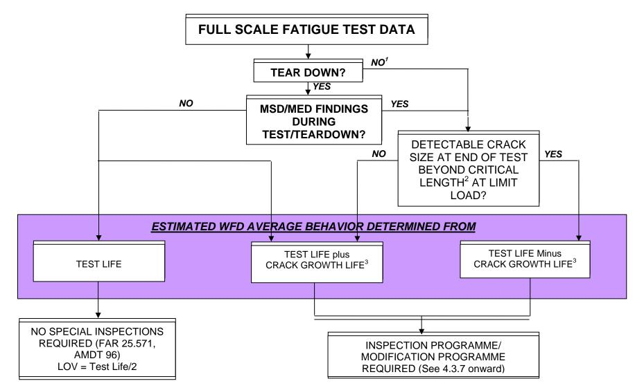
1 ASSUMED STATE AT END OF TEST: Best estimate of non-detected damage from inspection method used at end of test or during teardown.
