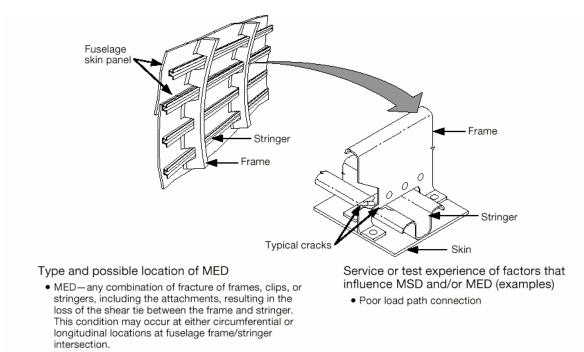
Figure A2-5 Stringer to Frame Attachments (MED)
