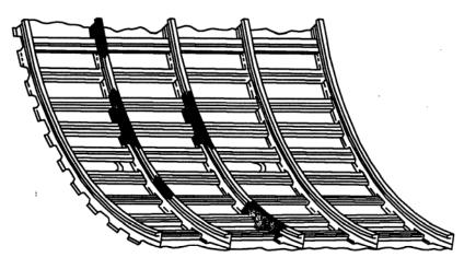
WIDESPREAD CORROSION (Corrosion occurring in adjacent frames)
