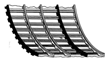
LOCAL CORROSION (Corrosion occurring in non-adjacent frames)
