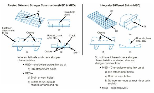
Figure A2-16 Typical Wing and Empennage Construction (MSD/MED)
