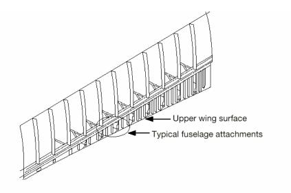
Type and possible location of MSD/MED • MED-repeated details in overwing fuselage attachments Service or test experience of factors that influence MSD and/or MED (examples)
