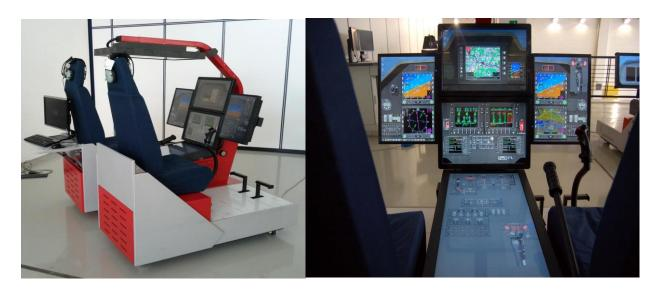
The touch-screen monitor display a graphical interactive and dynamic representation of the cockpit panels, controls, indicators and displays. The layout of the information displayed on the monitors is representative in terms of size, proportion and displacement, of the actual helicopter.
