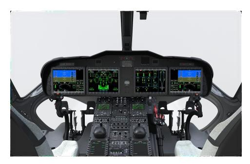
The instrument panel and inter-seat console contain all the control panels and displays governing the systems installed in the aircraft and utilised by the flight crew. The overhead console is installed above the heads of the flight crew and includes the circuit breaker panels and the rotor brake control lever.
