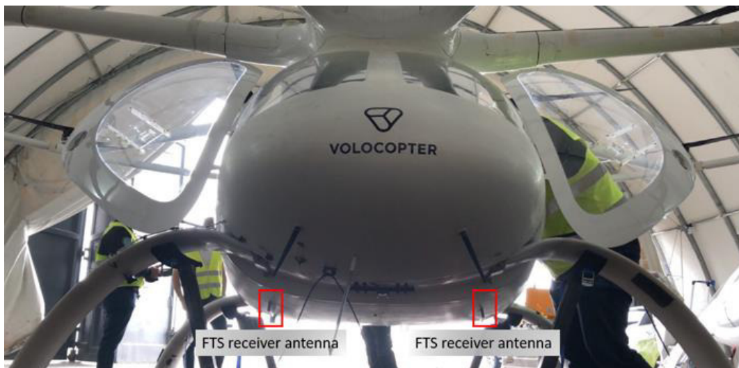
Fig. 3. – allocation of FTS onboard antennas on aircraft
