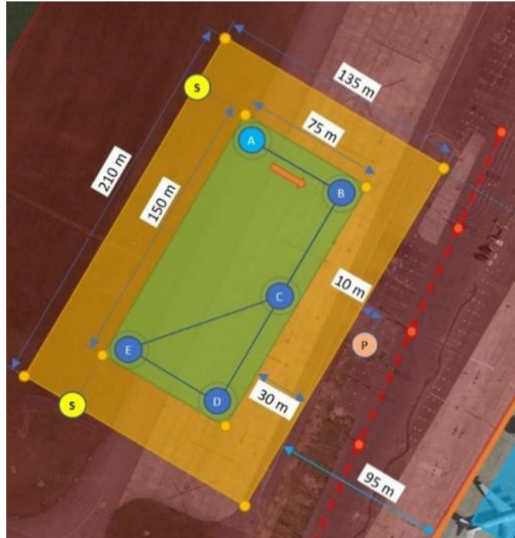
Fig. 11.- Operational Area (green and amber) and ground risk buffer (red). Pilot and FTS Operator are located at position "P".
