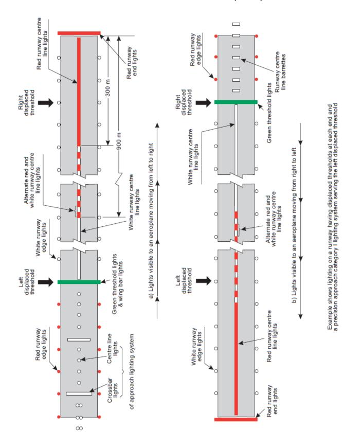
Figure M-8. Example of approach and runway lighting for runway with displaced thresholds
