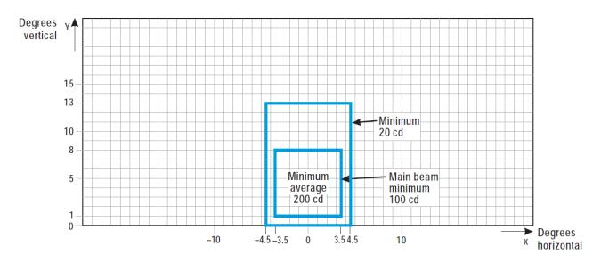
Figure U-17. Isocandela diagram for taxiway centre line (15 m spacing) and stop bar lights in straight sections intended for use in runway visual range conditions of less than a value of 350 m
