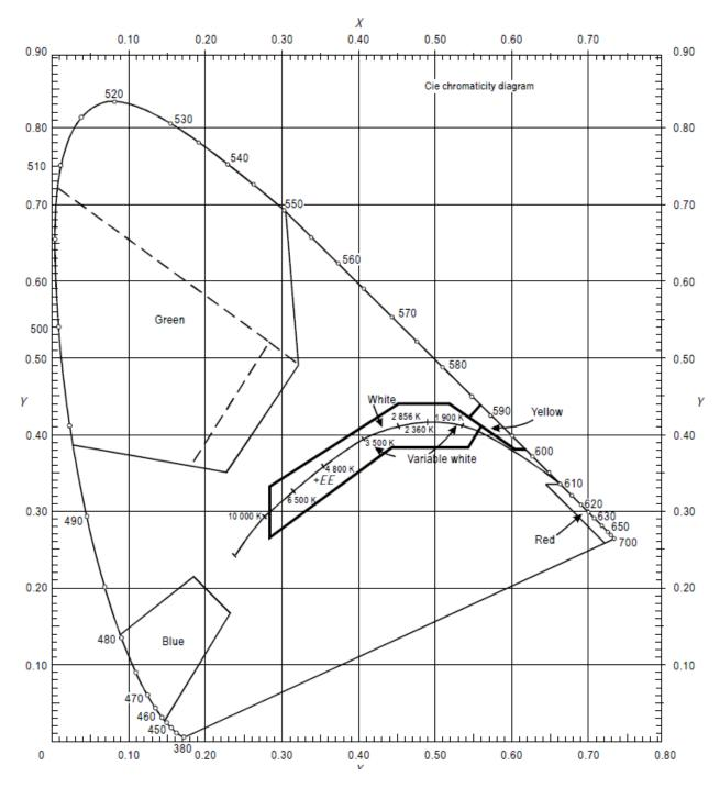
Figure U-1. Colours for aeronautical ground lights
