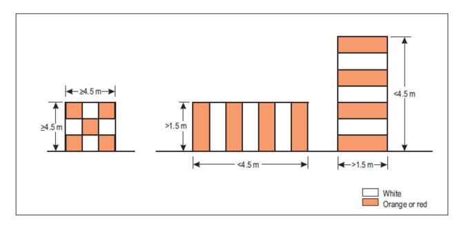
Figure Q-1. Basic marking patterns
