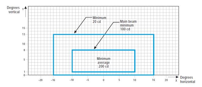
Figure U-16. Isocandela diagram for taxiway centre line (15 m spacing) and stop bar lights in straight sections intended for use in runway visual range conditions of less than a value of 350 m where large offsets can occur and for low-intensity runway guard lights, Configuration B
