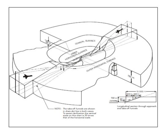
Figure GM-H-1 Disposition of Outer Horisontal Suface
