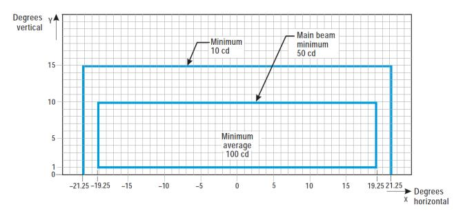
Figure U-18. Isocandela diagram for taxiway centre line (7.5 m spacing) and stop bar lights in curved sections intended for use in runway visual range conditions of less than a value of 350 m
