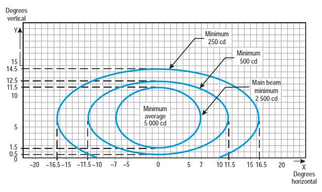
Figure U-6. Isocandela diagram for approach side row light (red light)
