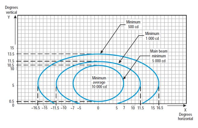
Figure U-8. Isocandela diagram for threshold wing bar light (green light)
