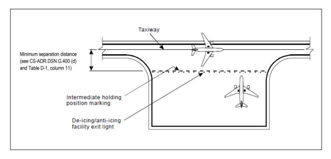
Figure M-11. Example of remote de-icing/anti-icing facility
