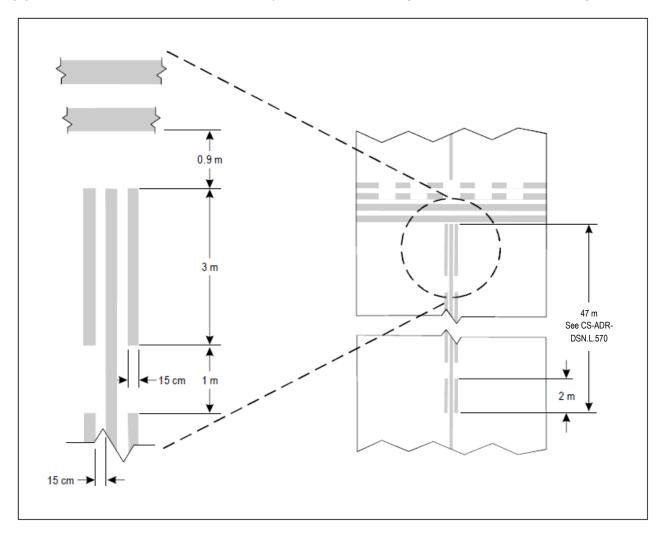
Figure L-6. Enhanced taxiway centre line marking
