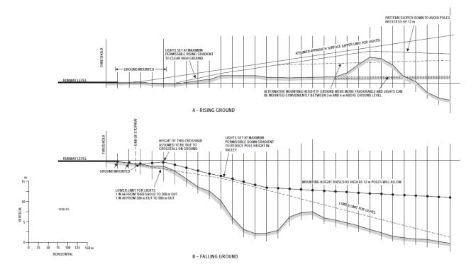
Figure GM-M-1. Vertical installation tolerances
