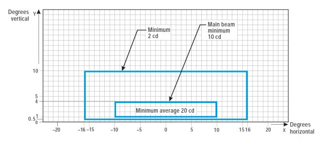
Figure U-19. Isocandela diagram for taxiway centre line (30 m, 60 m spacing) and stop bar lights in straight sections intended for use in runway visual range conditions of 350 m or greater
