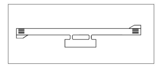
Figure GM B-3. Typical turn pad layout
