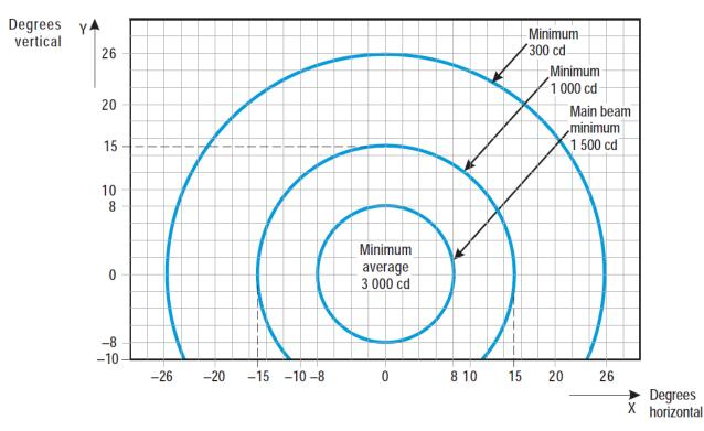
Figure U-28. Isocandela diagram for each light in high-intensity runway guard lights, Configuration A
