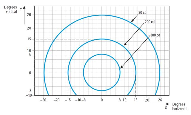
Figure U-27. Isocandela diagram for each light in low-intensity runway guard lights, Configuration A
