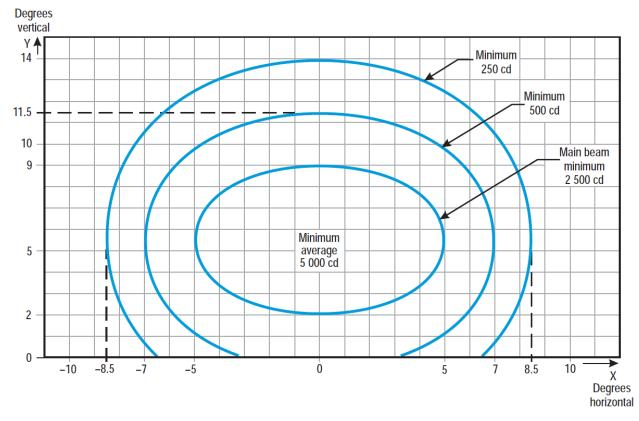
Figure U-9. Isocandela diagram for touchdown zone light (white light)
