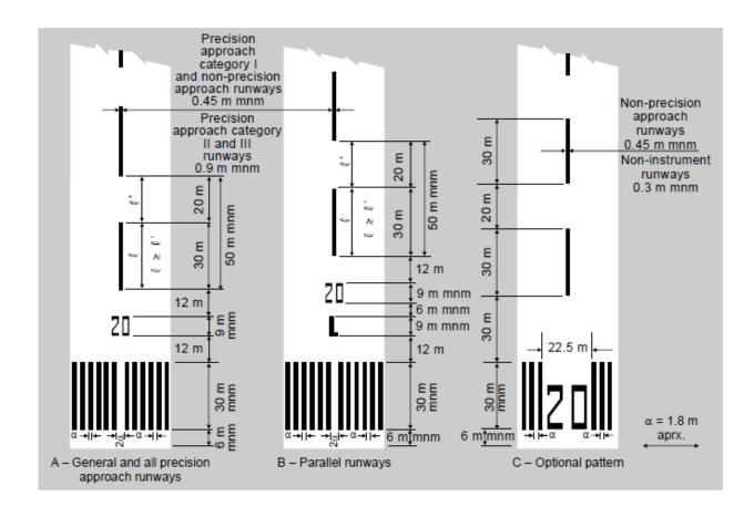
Figure L-1 Runway designation, centre line and threshold markings
