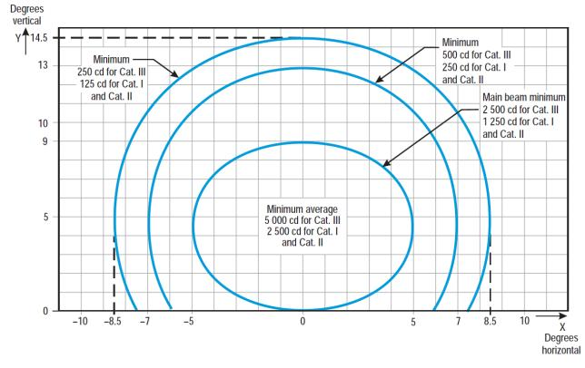
Figure U-11. Isocandela diagram for runway centre line light with 15 m longitudinal spacing (white light) and rapid exit taxiway indicator light (yellow light)
