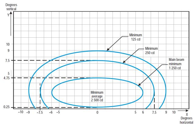
Figure U-12. Isocandela diagram for runway end light (red light)
