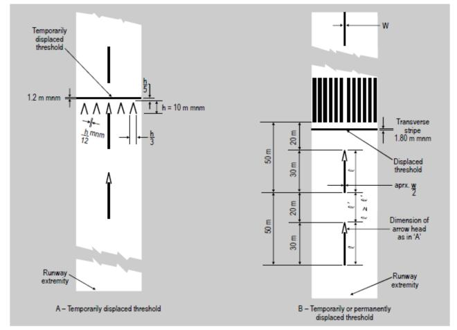
Figure L-3. Displaced threshold markings
