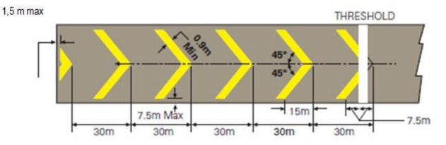
Figure R-2. Pre-threshold area marking
