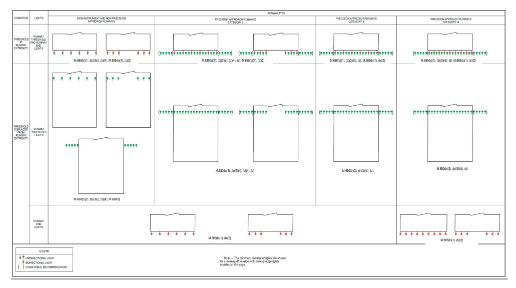
Figure M-7. Arrangement of runway threshold and runway end lights
