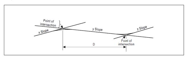
Figure GM-B-2. Profile on centre line of runway
