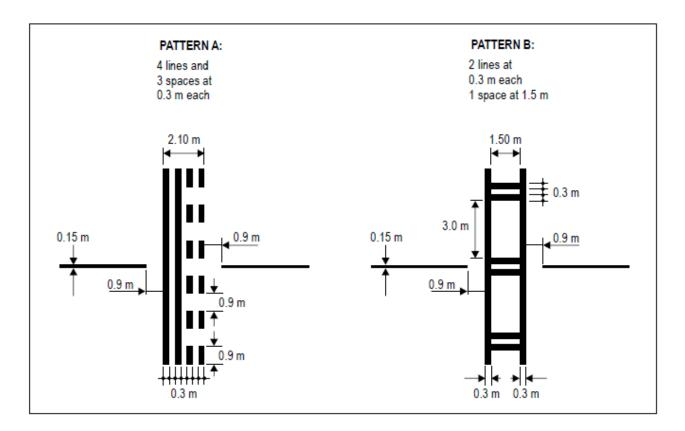
Figure L-7. Runway-holding position markings
