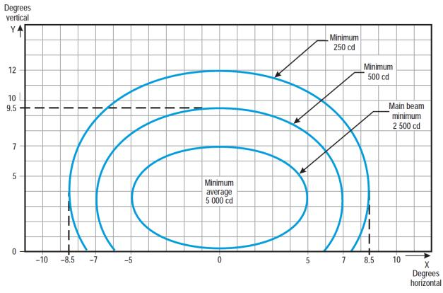
Figure U-10. Isocandela diagram for runway centre line light with 30 m longitudinal spacing (white light) and rapid exit taxiway indicator light (yellow light)
