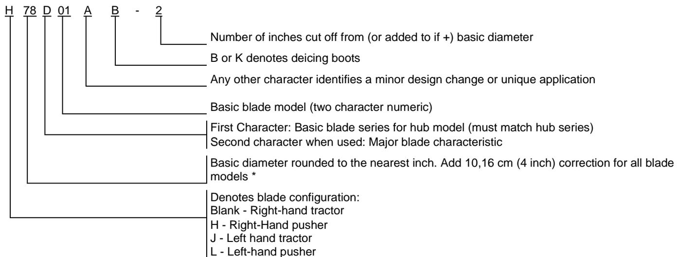
\*: Diameter limits are nominal diameters of the assembled propeller. They do not include the + or – 0,32 cm (1/8 inch) manufacturing tolerance the FAA allows for propeller with a basic diameter of less than 426,7 cm (14 feet).
