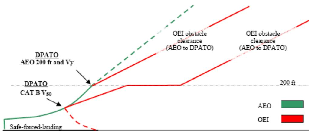
Otherwise, and if scheduled in the AFM, the AEO distance to 50 ft ( $V_{50}$ ) – determined in accordance with CS/JAR 29.63 – can be used (see Figure 7). Where this distance is used, it will be necessary to ensure that the  $V_{50}$  climb out speed is associated with a speed and mass for which OEI climb data is available so that, from  $V_{50}$ , the OEI flight path can be constructed.
