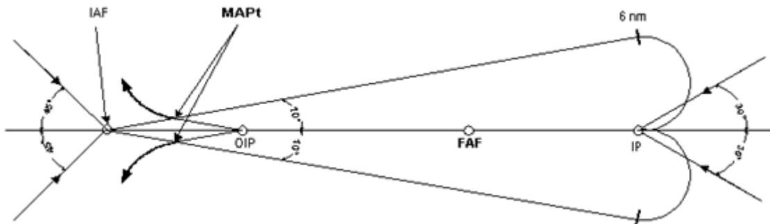
**Figure 3: Holding pattern & race track procedure**
