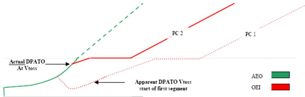
The apparent DPATO is for planning purposes only in the case where AEO data are not available to construct the take-off flight path. The actual OEI flight path will provide better obstacle clearance than the apparent one (used to demonstrate the minimum requirement) - as seen from the firm and dashed lines in the above figure.
