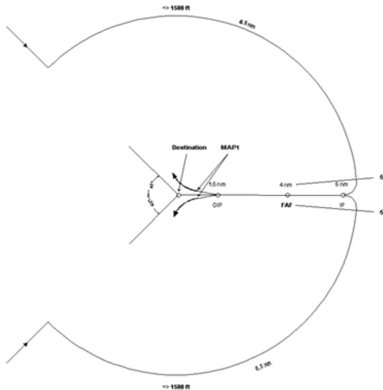
**Figure 2: Base turn procedure – direct approach**
