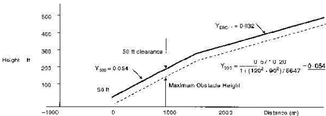
(2) Assumed engine failure height 200 ft
