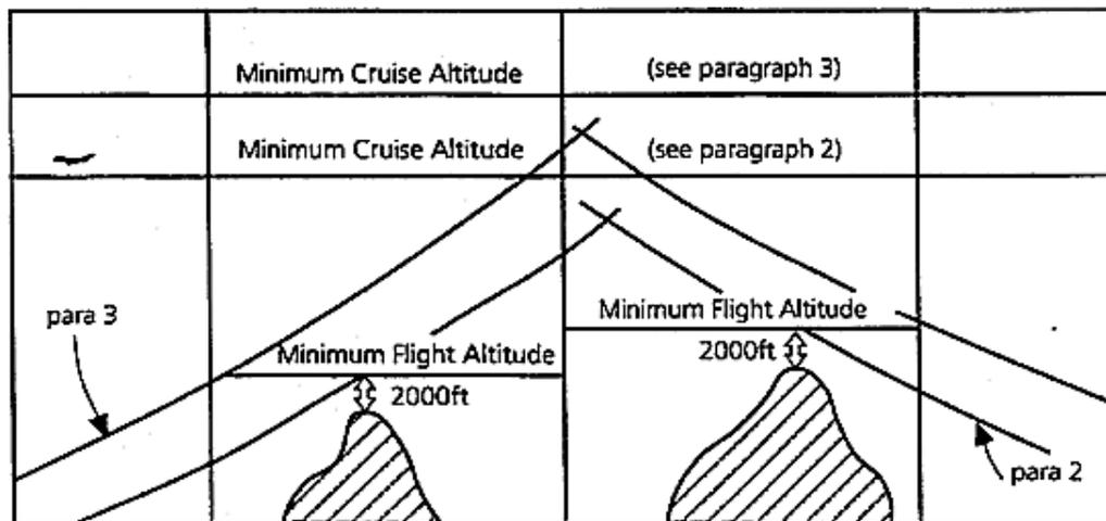
Note: MEA or MORA normally provide the required 2 000 ft obstacle clearance for driftdown. However, at and below 6 000 ft altitude, MEA and MORA cannot be used directly as only 1 000 ft clearance is ensured.
