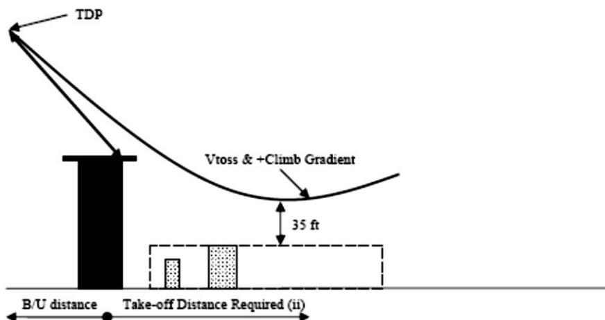
The main difference is that drop down below the level of the take-off surface is permitted. In the drop down phase, the Category A procedure ensures deck-edge clearance but, once clear of the deck-edge, the 35 ft clearance from obstacles relies upon the calculation of drop down. Item (b) of AMC1 CAT.POL.H.205(b)(4) is applied.
