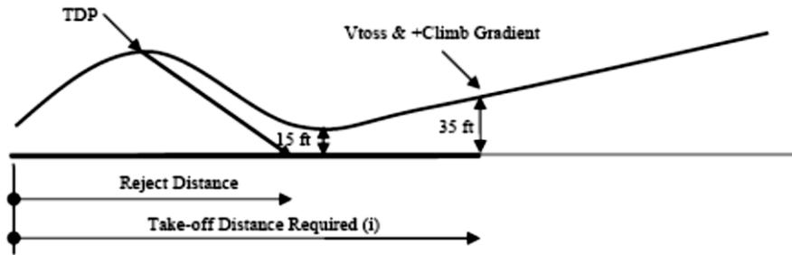
The operator only has to establish that the distances required are within the distance available (take-off distance and reject distance). The original definition of TODRH meets this case exactly.
