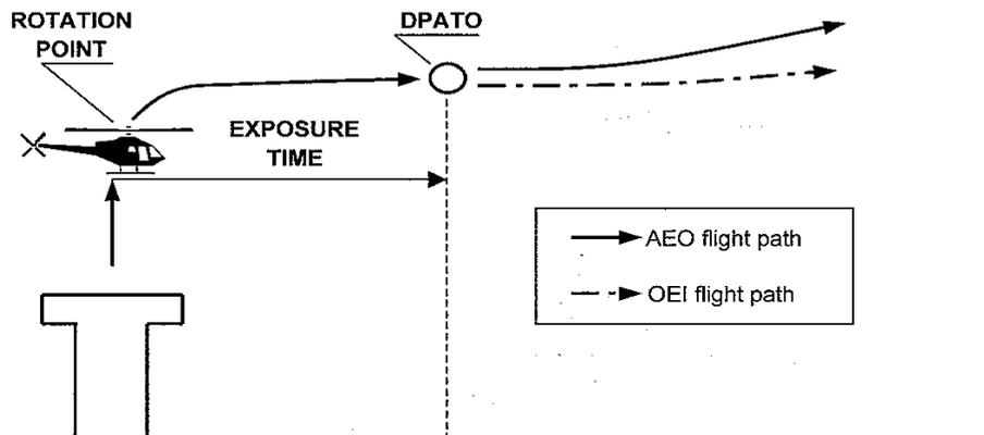
(f) Landing - non-hostile environment (without an approval to operate with an exposure time) CAT.POL.H.325 (b)
