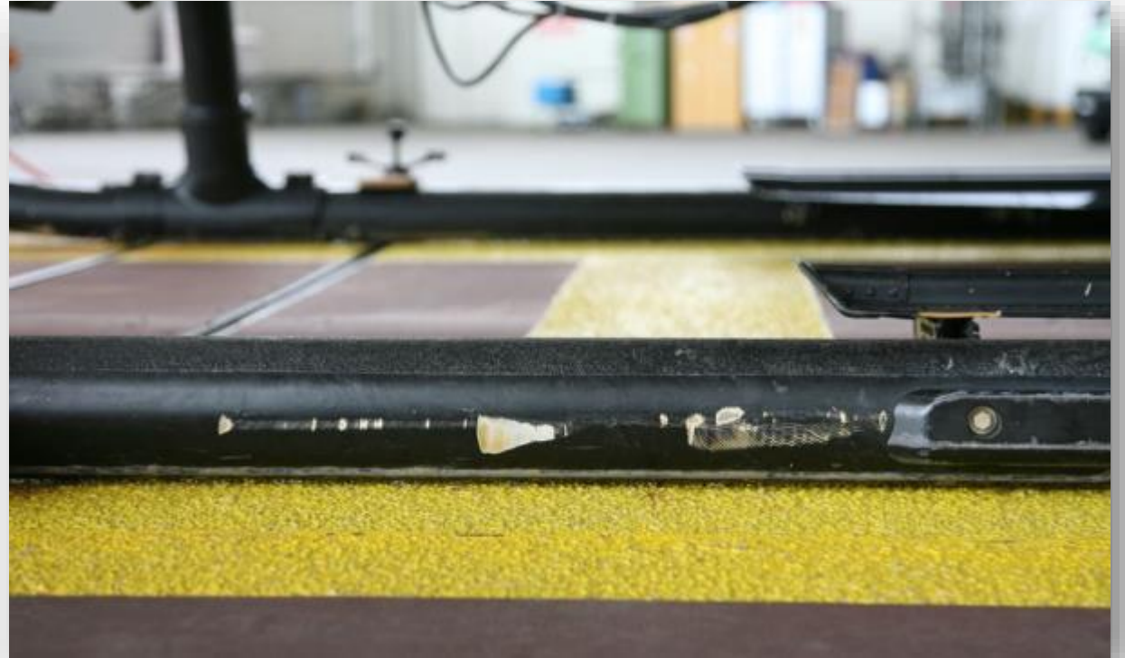
Cable Chafing on Landing Gear Skid Tube
