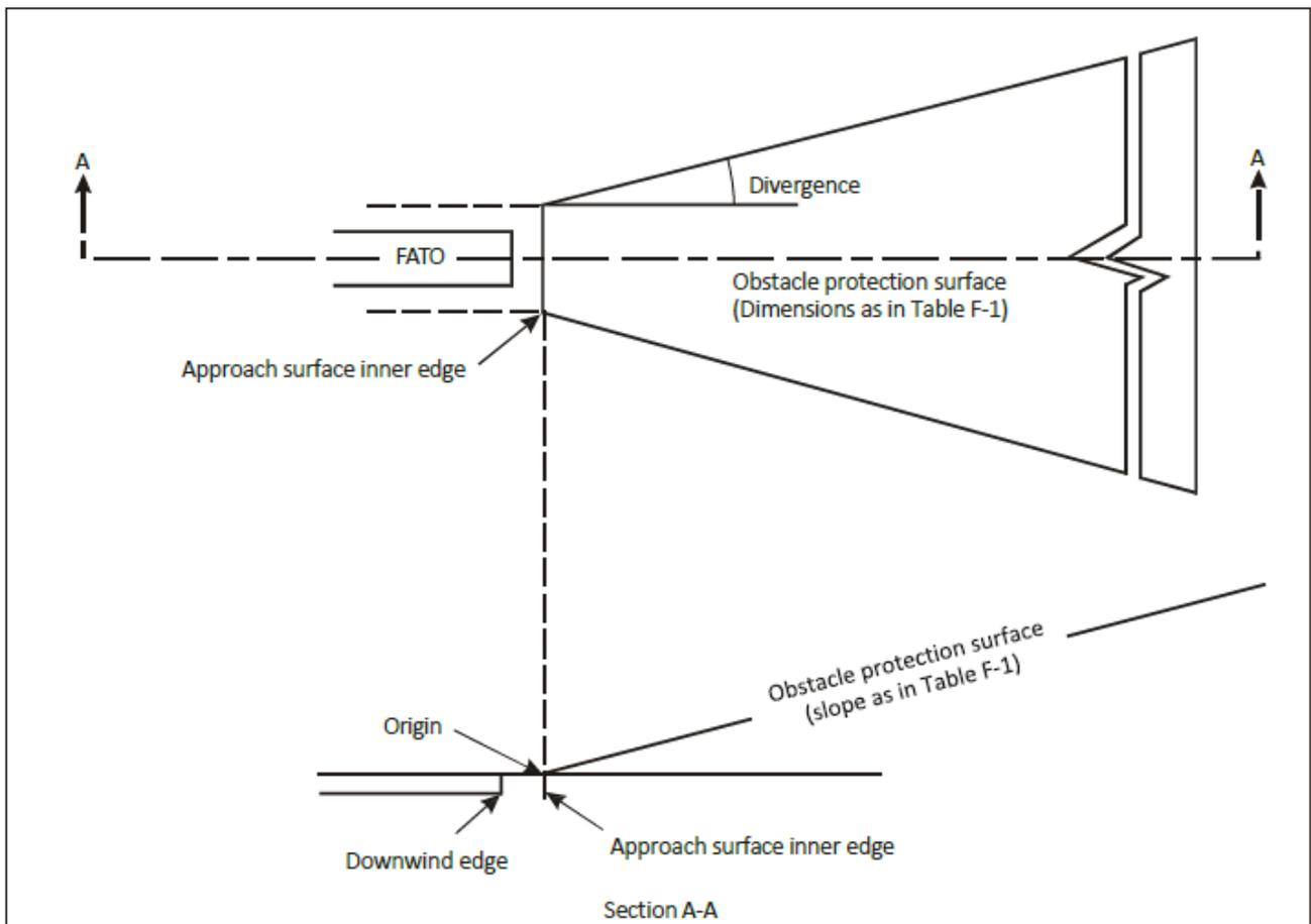
Figure F-7. Obstacle protection surface for visual approach slope indicator systems
