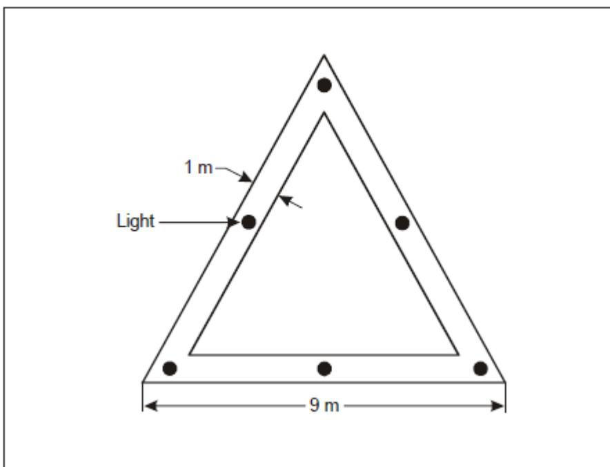
Figure F-9. Aiming point marking and lighting
