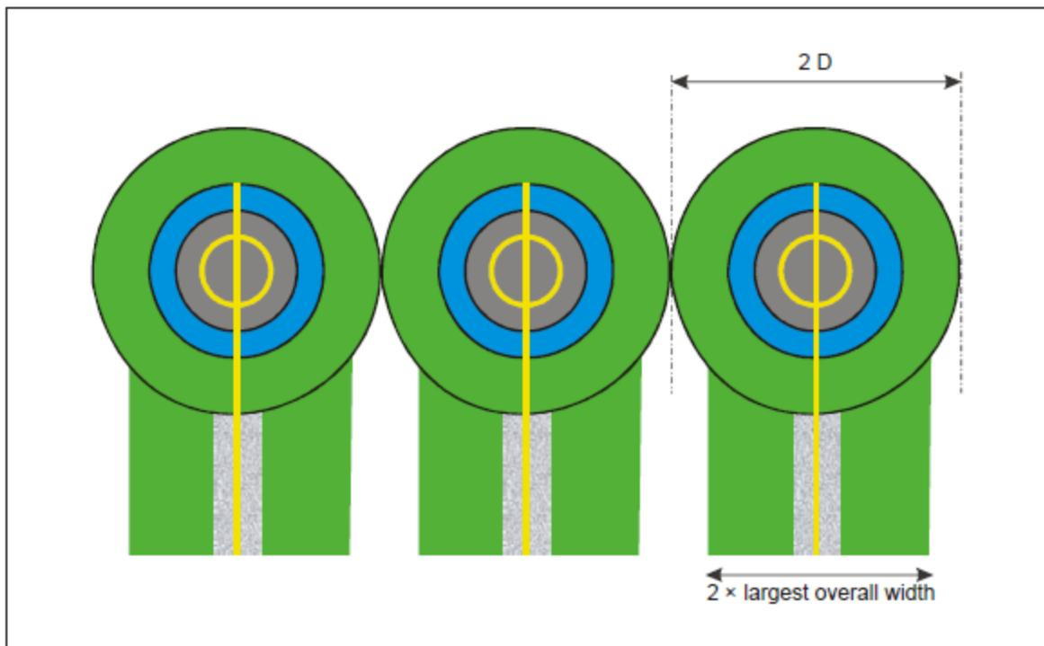
Figure D-2. Helicopter stands designed for hover turns with air taxi-routes/taxiways — simultaneous operations
