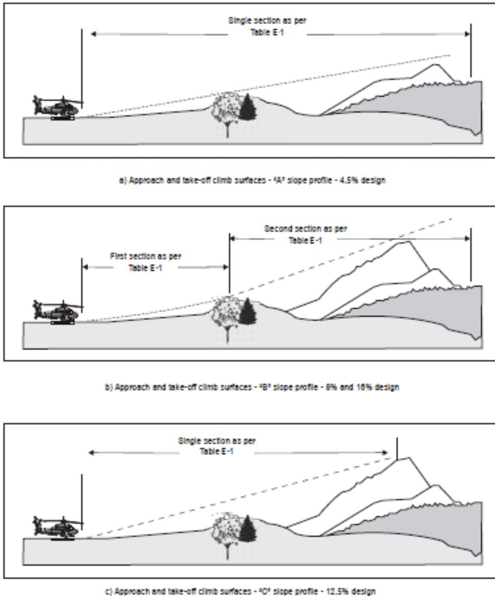
Figure E-4. Approach and take-off climb surfaces with different slope design categories
