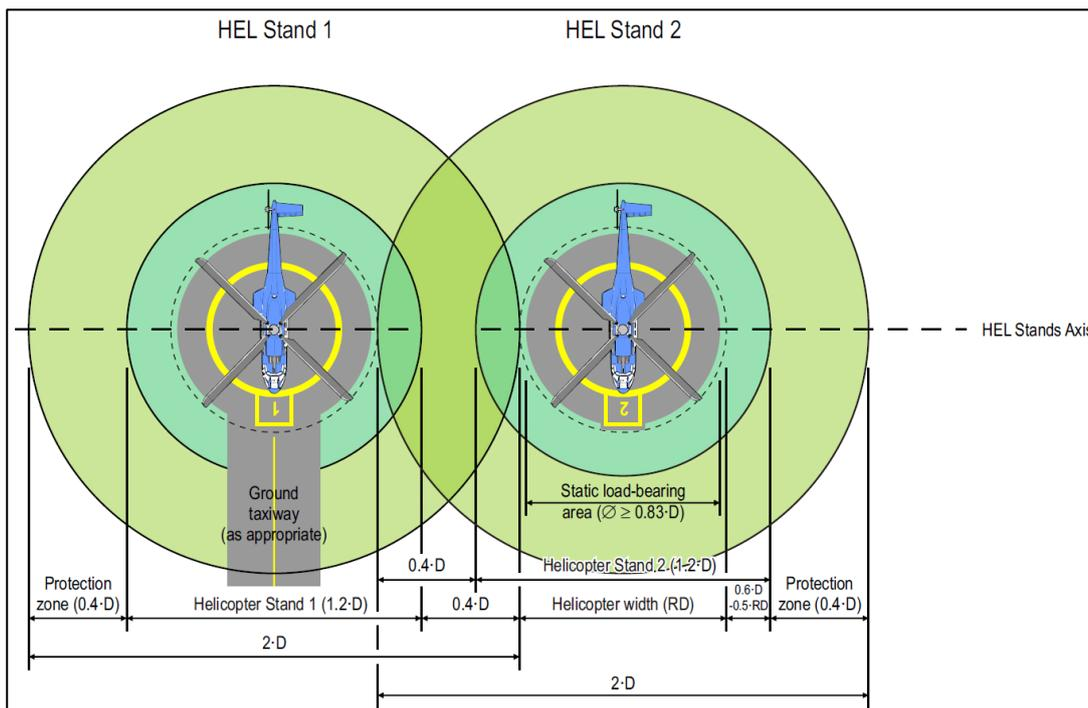
Figure GM D-1. Reduced separation distance between helicopter stands
