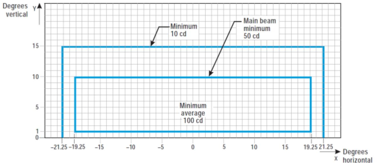
Figure U-18. Isocandela diagram for taxiway centre line (7.5 m spacing), no-entry bar, and stop bar lights in curved sections intended for use in runway visual range conditions of less than a value of 350 m
