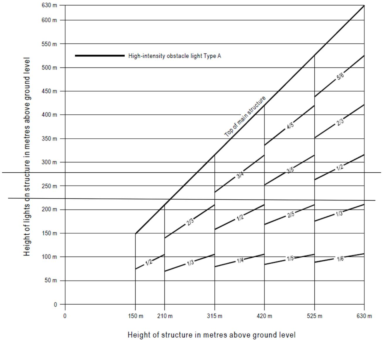
Figure GM-Q-6. High-intensity flashing white obstacle lighting system, Type A
