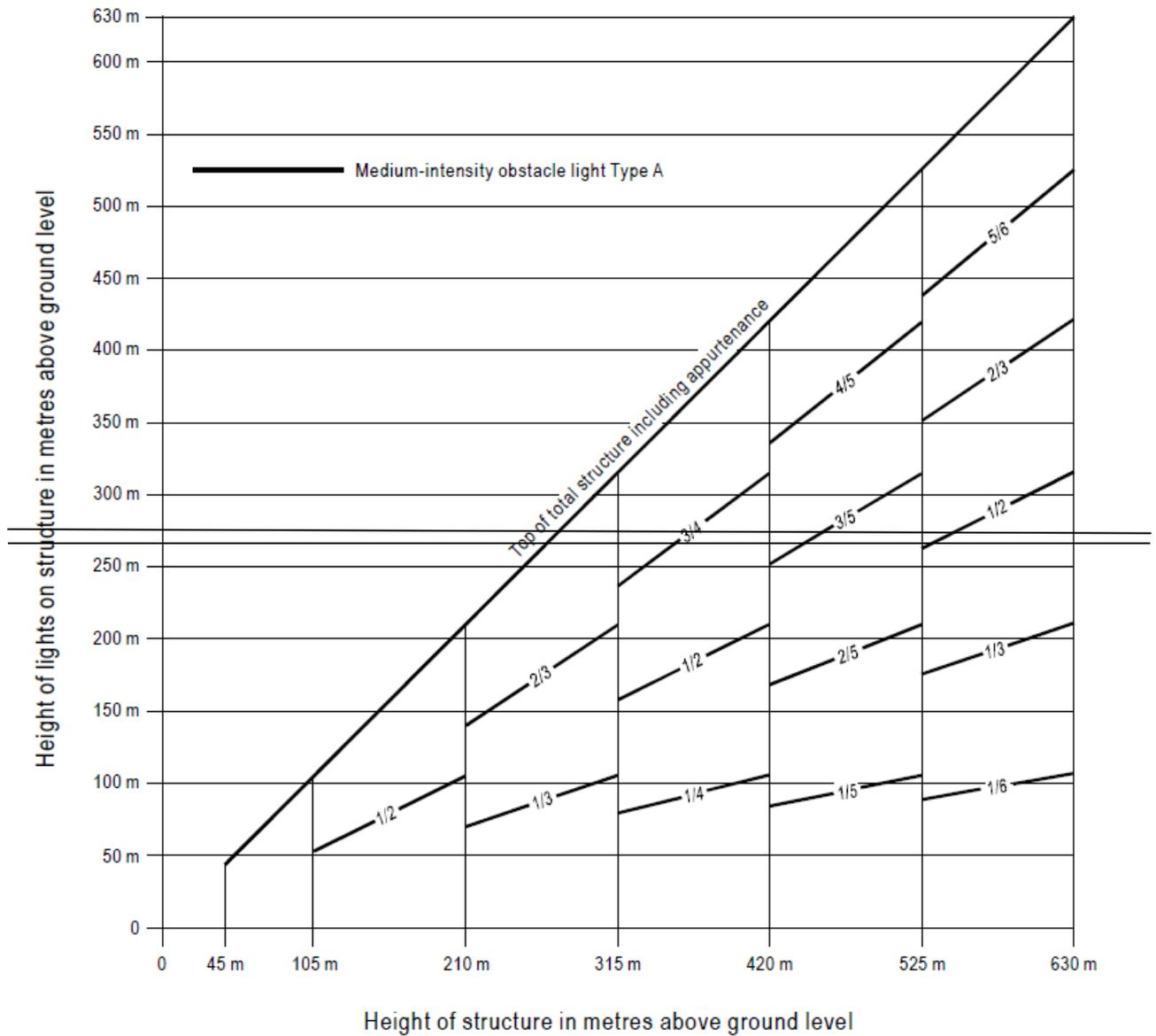
*Note.— High-intensity obstacle lighting is recommended on structures with a height of more than 150 m above ground level. If medium-intensity lighting is used, marking will also be required.*
