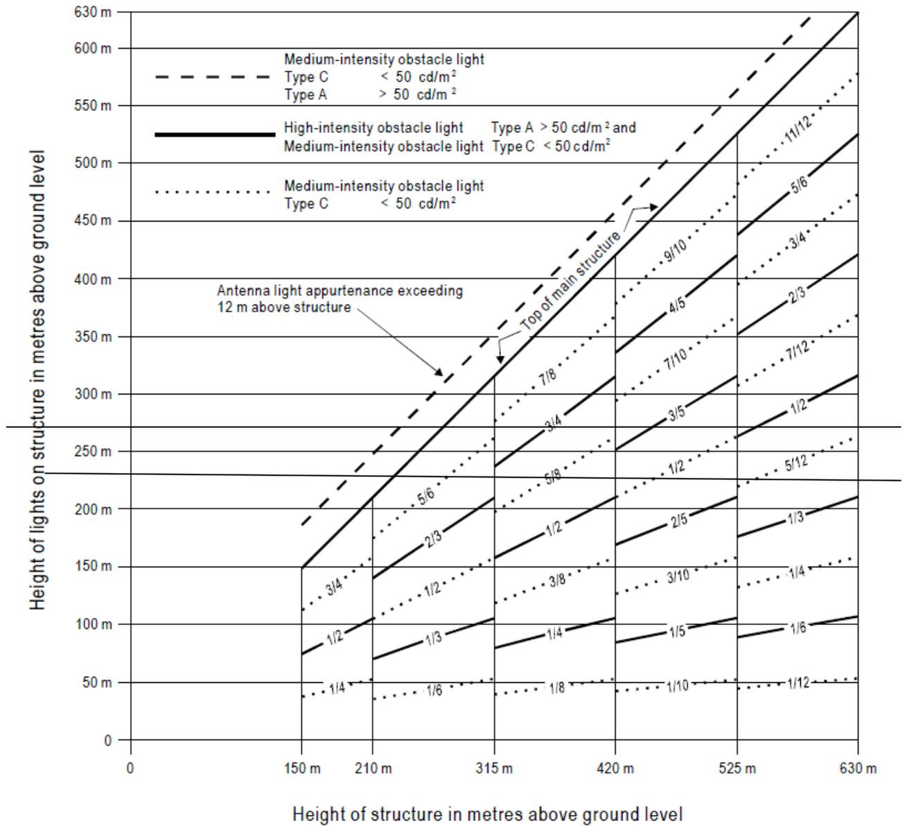
Figure GM-Q-8. High-/medium-intensity dual obstacle lighting system, Type A/Type C
