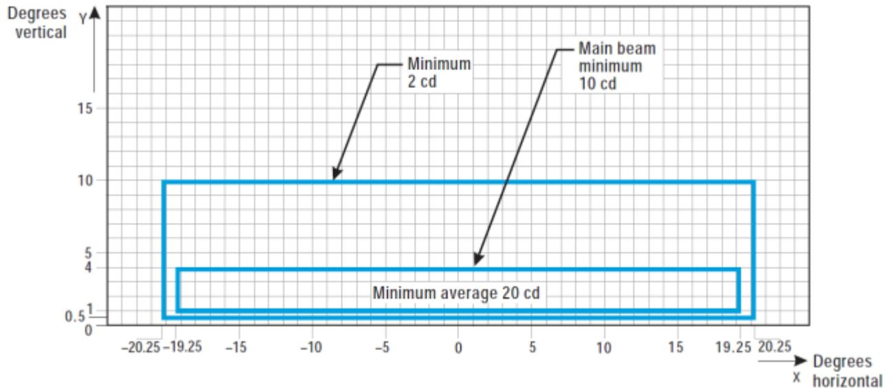
Figure U-20. Isocandela diagram for taxiway centre line (7.5 m, 15 m, 30 m spacing), no-entry bar, and stop bar lights in curved sections intended for use in runway visual range conditions of 350 m or greater
