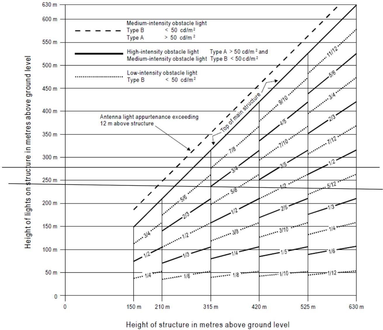
Figure GM-Q 7. High /medium intensity dual obstacle lighting system, Type A/Type B
