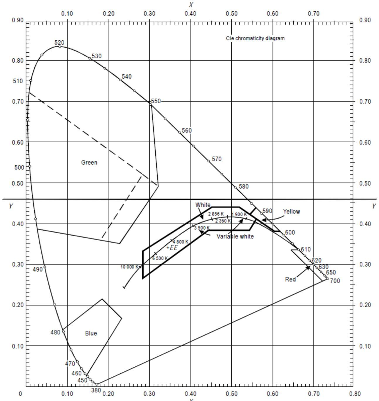
Figure U-1. Colors for aeronautical ground lights
