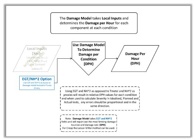
Figure 8.12 — EGT Method Damage Model
