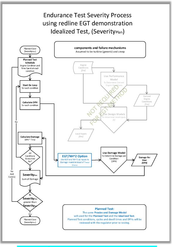
Figure 8.10 — Endurance Test Severity Process using RL EGT Demonstration — Idealised Test (Severity<sub>Plan</sub>)
