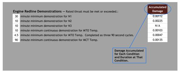
Figure 7.2 — Severity Usage for Engine Redline Demonstrations
