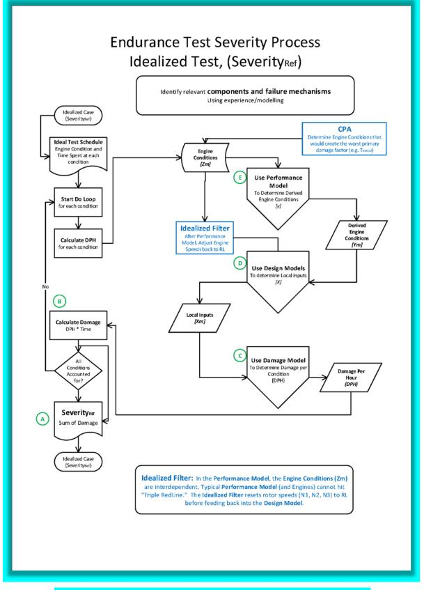
Figure 8.3 — Endurance Test Severity Process — Idealised Test (Severity<sub>Ref</sub>)
