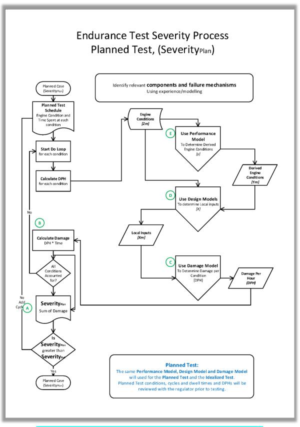
Figure 8.4 — Endurance Test Severity Process — Planned Test (Severity<sub>Plan</sub>)
