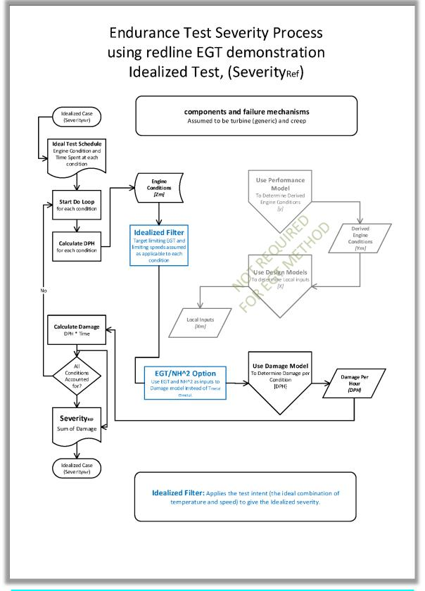
Figure 8.9 — Endurance Test Severity Process using RL EGT Demonstration — Idealised Test (Severity $_{\mathsf{Ref}}$ )
