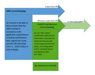
\*: Transmitted records is a subset of AMO maintenance records provided to the CA(M)O. Certain transmitted records do not need to be kept as a record by the CA(M)O such as EASA Form 1 for a component with no scheduled maintenance task selected and not subject to AD or modification/repair.
