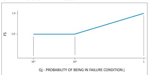
Figure 3: Factor of safety for continuation of flight
