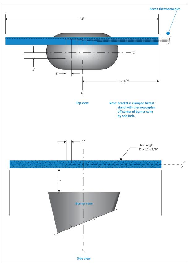
FIGURE 3 THERMOCOUPLE RAKE BRACKET
