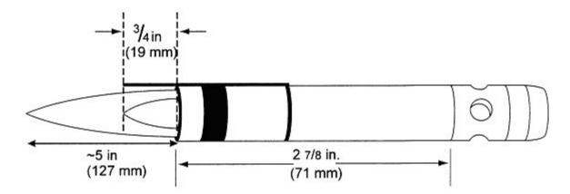
Figure 6 - Propane Pilot Burner
