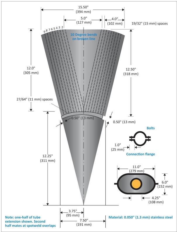
Figure 3 – Burner Draft Tube Extension Cone Diagram
