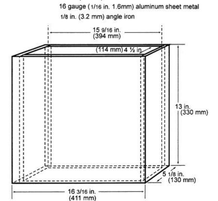
Figure 2 - Internal Chimney
