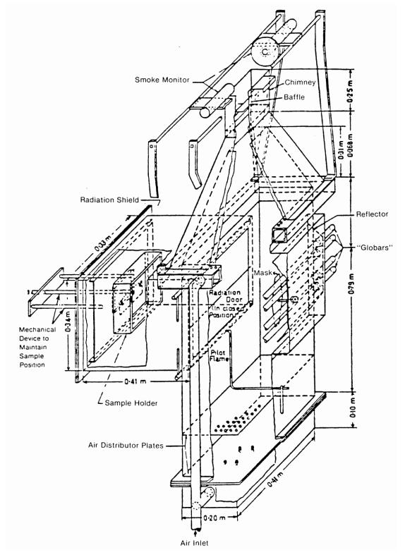
FIGURE 1. RELEASE RATE APPARATUS
