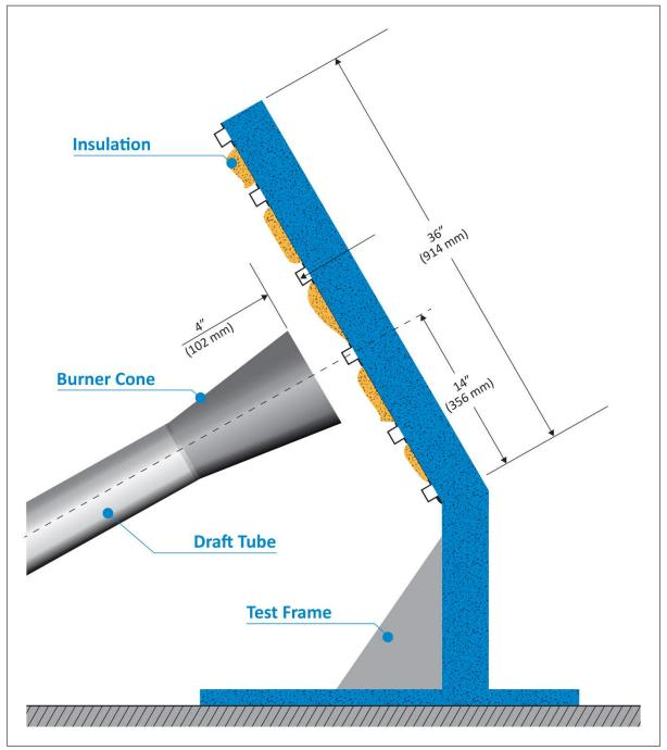
Figure 2 – Burnthrough Test Apparatus
