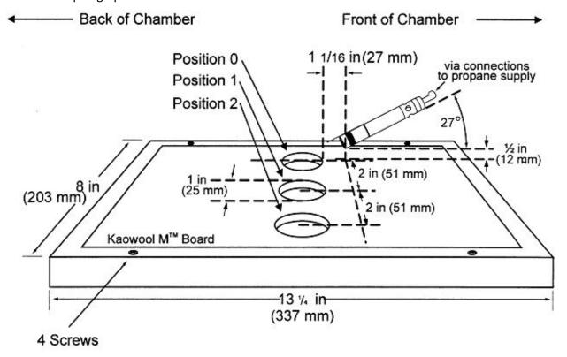
Figure 7 - Calorimeter Holding Frame
