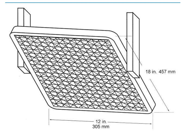
Figure 3b – Air Propane Radiant Panel
