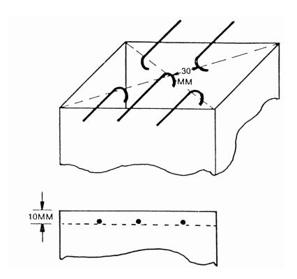
FIGURE 5. THERMOCOUPLE POSITION
