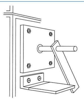
Figure 8 - Propane Burner Stop
