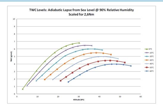
It is commonly recognised that below -40°C no liquid conditions exist anymore. Therefore testing in mixed phase conditions does not need to consider temperatures below -40°C.
