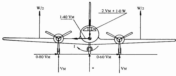
VM = One-half the maximum vertical ground reaction obtained at each main gear in the level landing conditions.
