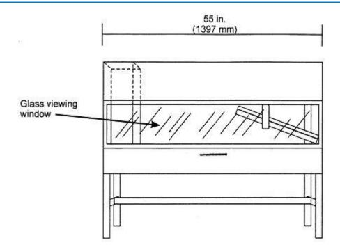
Figure 1 - Radiant Panel Test Chamber
