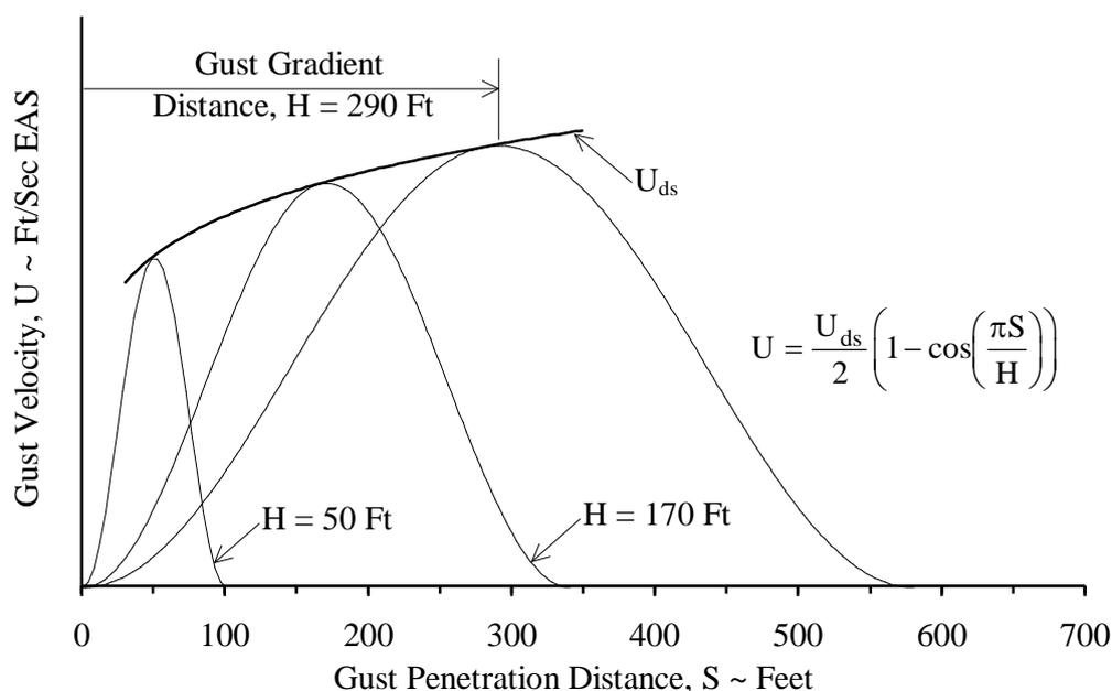
Figure-2 Typical (1-cosine) Design Gust Velocity Profiles
