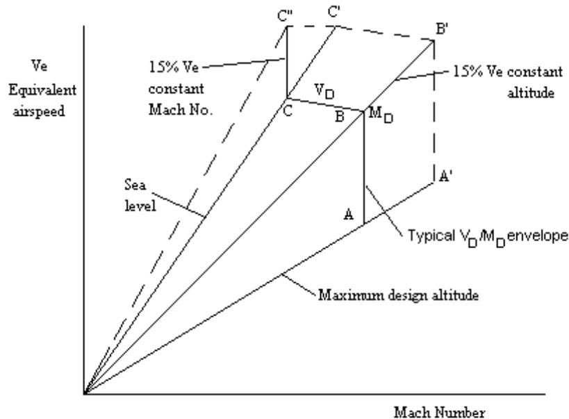
FIGURE 1B MINIMUM FAIL-SAFE CLEARANCE ENVELOPE
