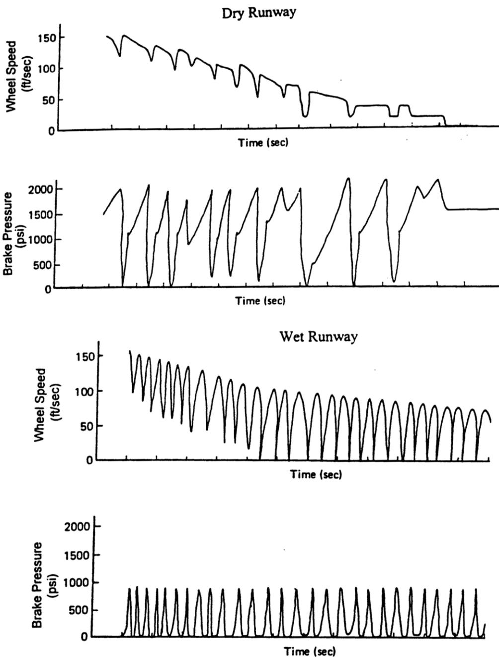
FIGURE 2. ANTI-SKID SYSTEM RESPONSE CHARACTERISTICS
