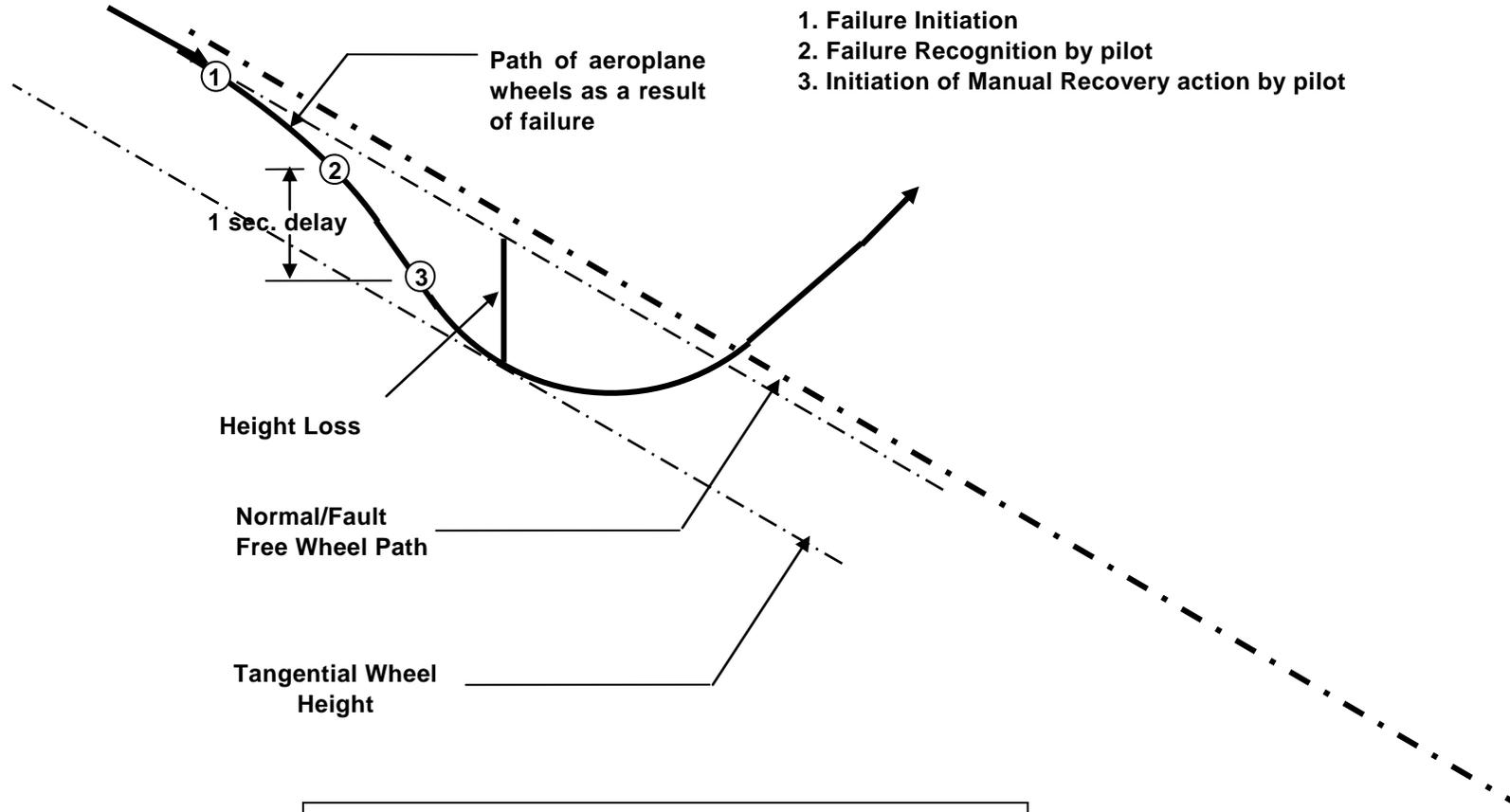
**Figure FT-2: Height Loss Method**
