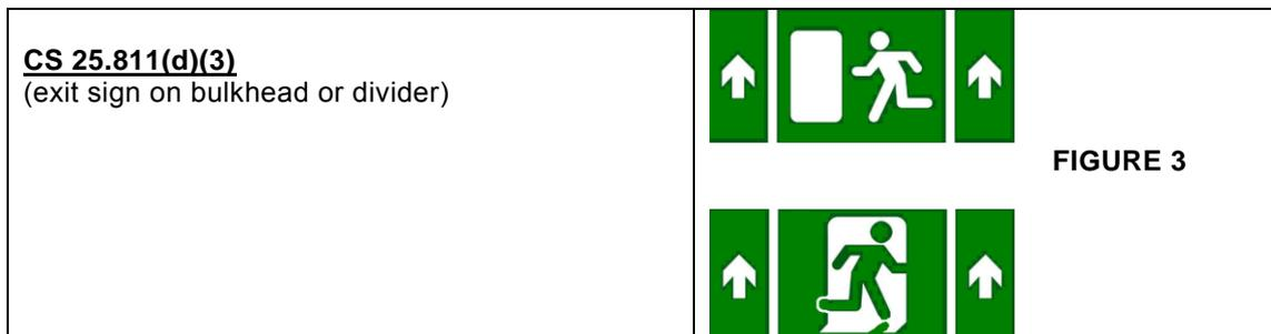
The design of symbolic exit signs should be chosen to provide a consistent set throughout the cabin.
