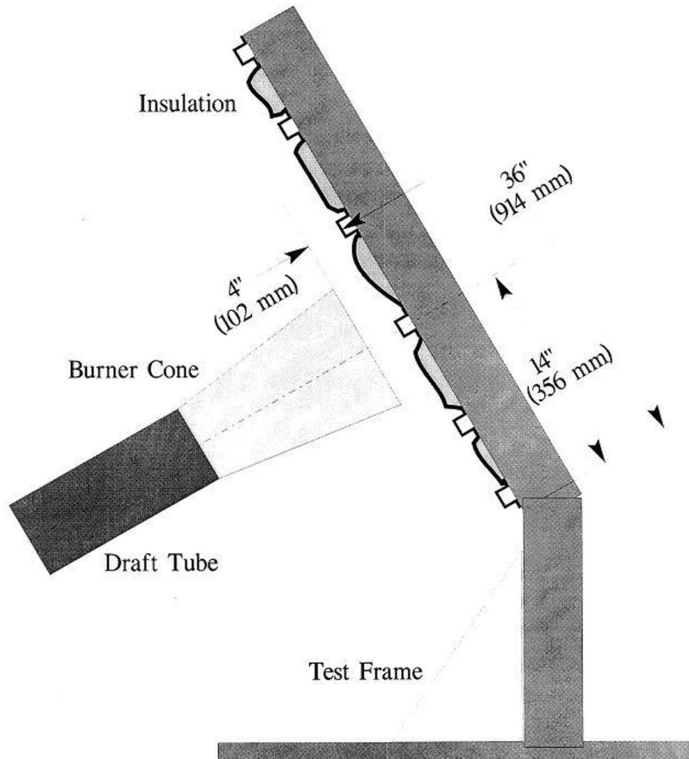
Figure 2 – Burnthrough Test Apparatus
