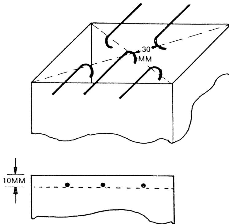
FIGURE 5. THERMOCOUPLE POSITION
