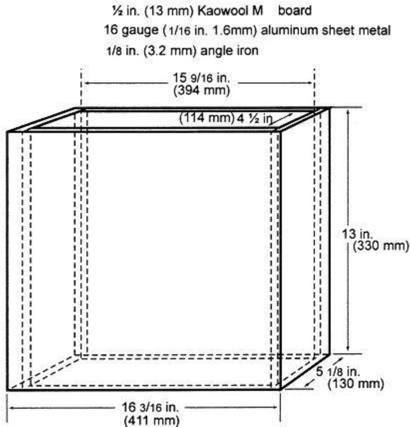
Figure 2 - Internal Chimney
