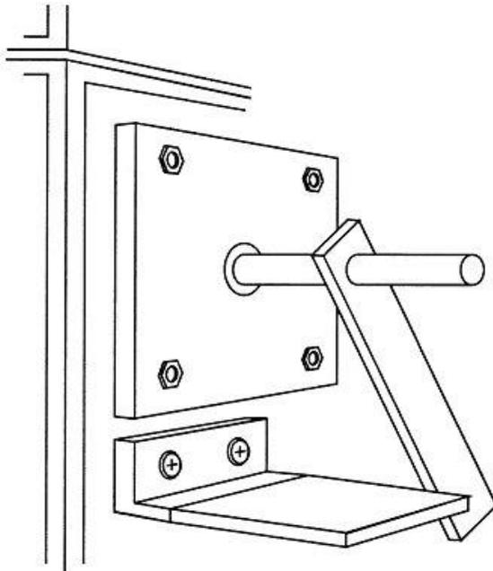
Figure 8 - Propane Burner Stop
