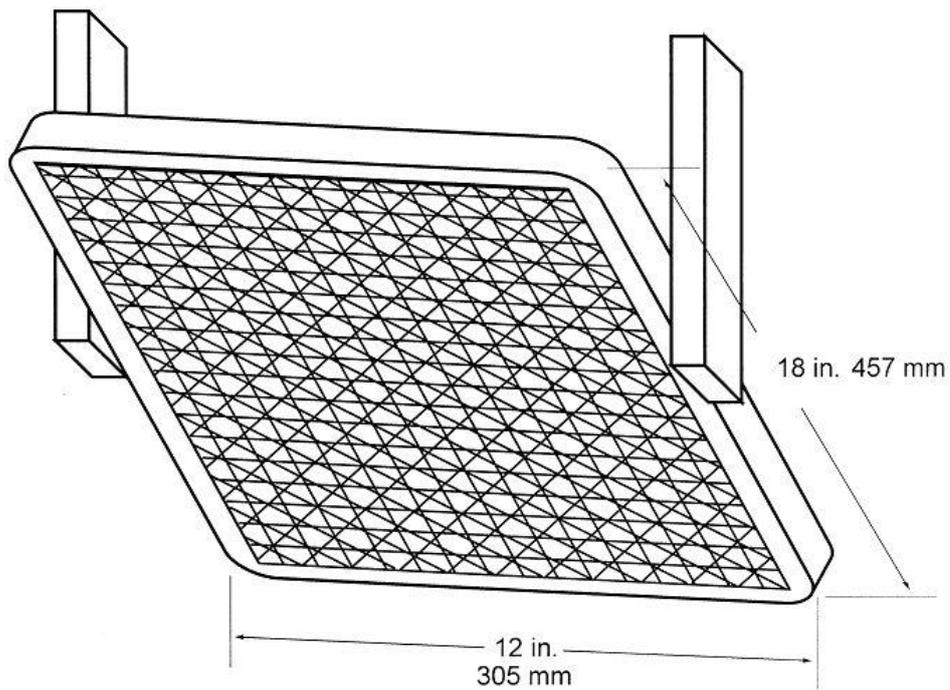
Figure 3b – Air Propane Radiant Panel
